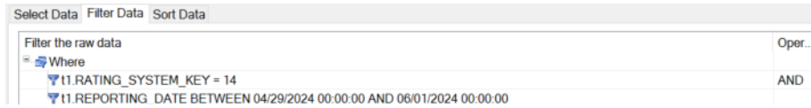
FIGURE 4.2: Filtering on the fact table with RATING_SYSTEM_KEY = 14 selects only the large corporate customers and REPORTING_DATE on April and May 2024
