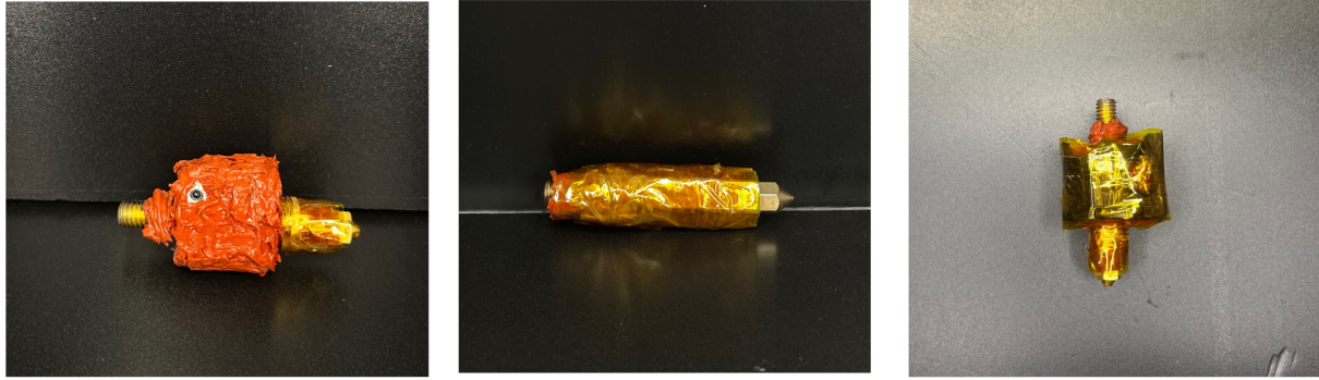
Figure 2.8 Illustration of nozzle heating and insulation process (A) Application of silicone glue (B) Nozzle extension without adding second heater block (C) Nozzle extension after adding second heater block
