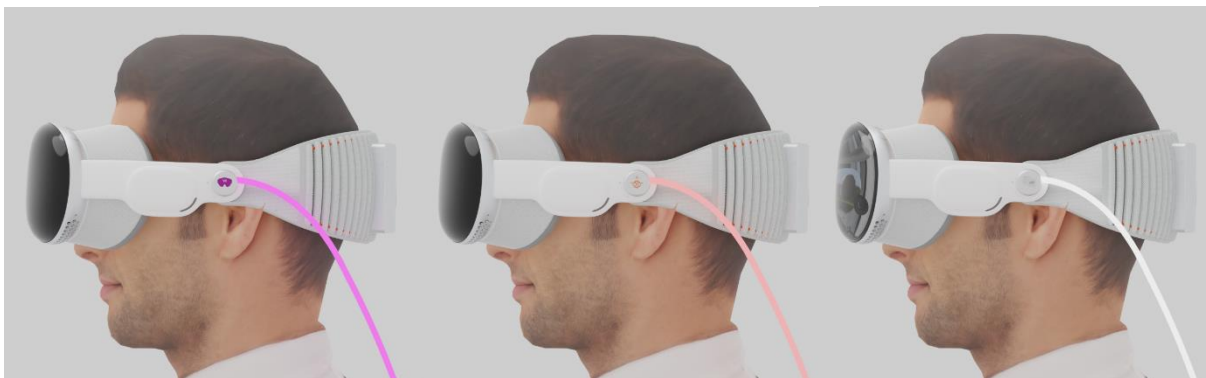
Figures 17, 18 & 19 – Close-up to see the VR-mode, AR-mode and OFF-mode indicators on the LED display and in the battery wire.
