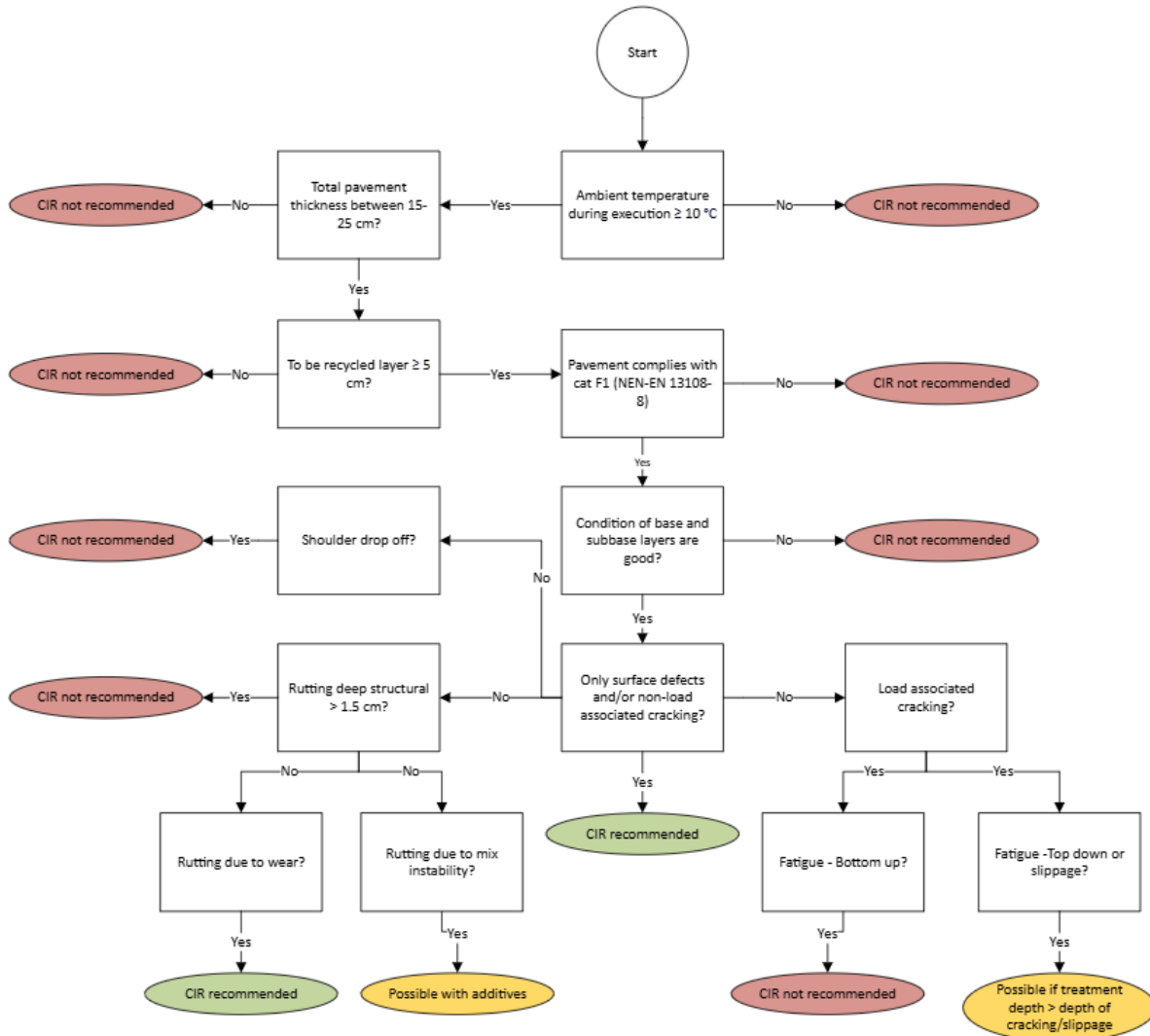
Figure E.1: Guideline for CIR project selection in the form of a flowchart
