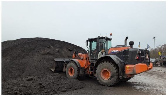
((a)) Shovel loader used to prepare the RAP stockpiles for sample collection
