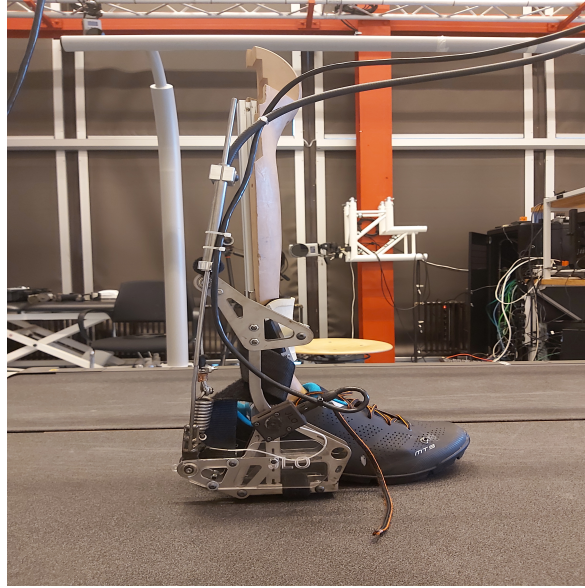
Figure 4.2: Positioning of the exoskeleton during experiments to determine the motor-side stiffness.
