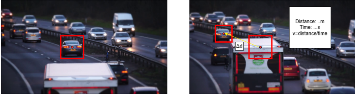
Figure 12: Speed estimation between frames
