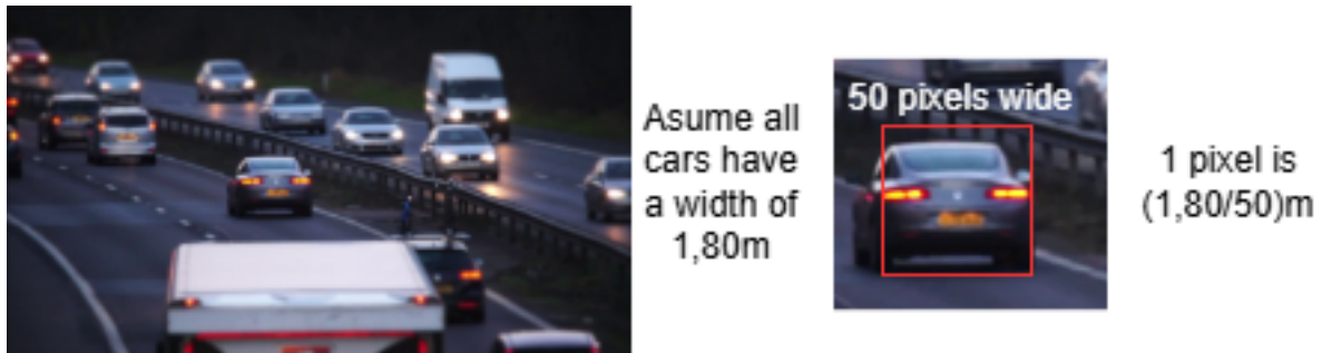
Figure 8: Standardized object scaling
