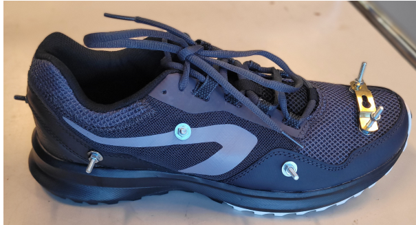
Figure 1. Provided neutral running shoe with metal fixture for the forefoot IMU and screws to fixate the lateral optical markers on the foot.
