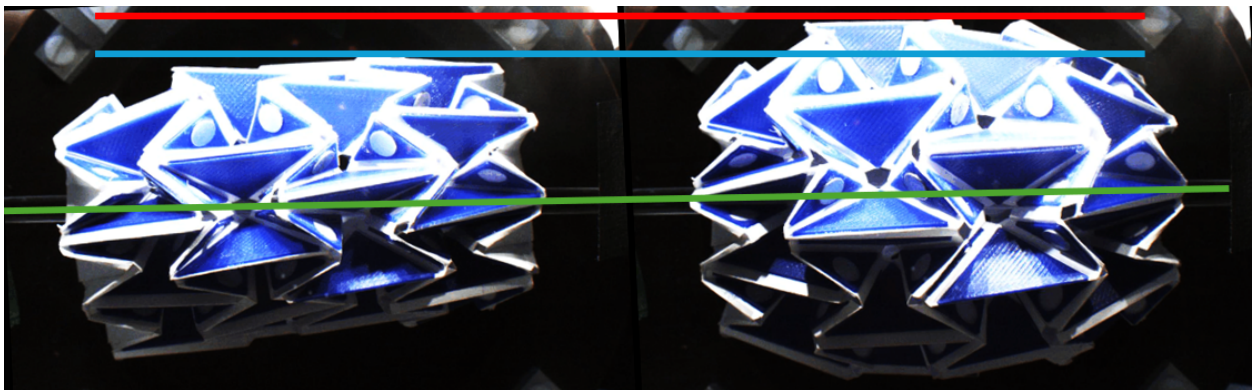
Figure 35: Frames of RM module being both collapsed and expanded during the quasi-static input experiment. Green: Baseline, Blue: maximum retraction, Red: maximum expansion
