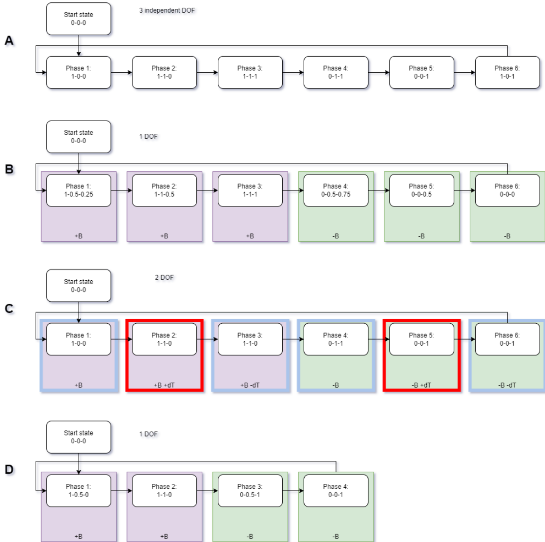
Figure 15: Explored locomotion sequences. (a) Ideal sequence. (b) First 1 DOF sequence (c) 2 DOF sequence (d) Second 1 DOF sequence
