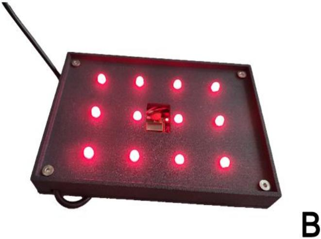
**Appendix 1.** PBMT Device. (A) shows the device on top of a 16 well plate and (B) shows the LED array side to be exposed to the 16 well plate.
