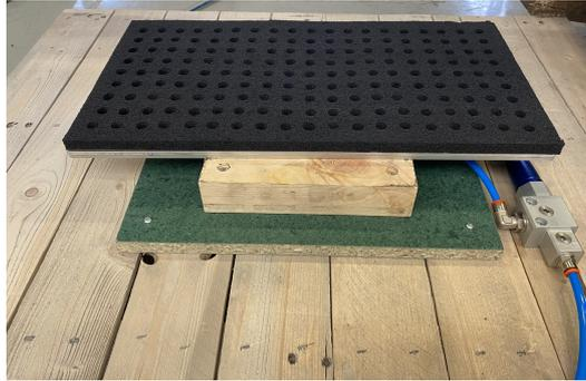
Figure 5.2: Fixture device that uses a 50 cm by 25 cm vacuum pad and can be used to fix a product in place and prevent sticking.
