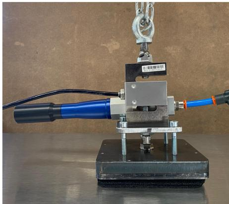
Figure 5.1: Destacking device that uses a 11.5 cm by 11.5 cm vacuum pad and can be used to measure and log the pulling force over time.
