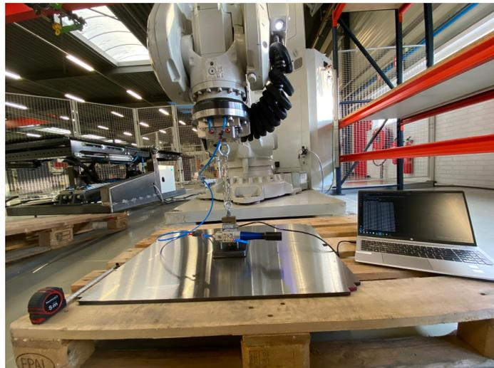
Figure 5.3: Experimental setup including the robotic manipulator, the test product, the destacking device from Figure 5.1 and a laptop for logging measured values.
