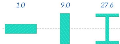
Figure 2.18: Area moment of inertia  $I$  for three different beam cross-sections [13].
