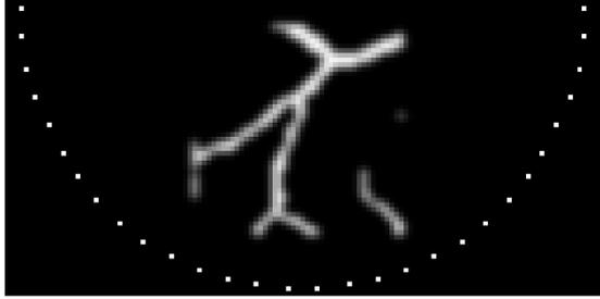
Figure 4.1: An initial pressure representing blood vessels is placed in the centre of a rectangular domain and is surrounded by a half-ring of perfect point-like ultrasound detectors.
