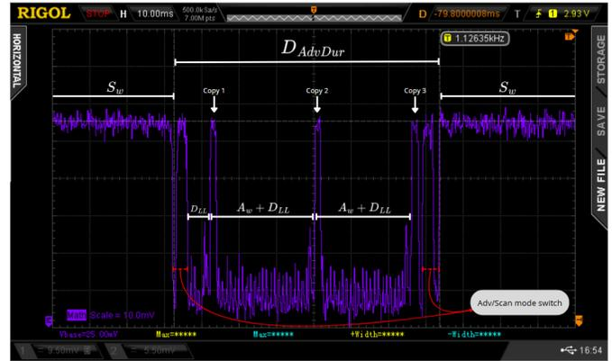
Fig. 18: Oscilloscope screenshot from a full advertising duration ( $S_w = 50$ ,  $N = 3$ ).
