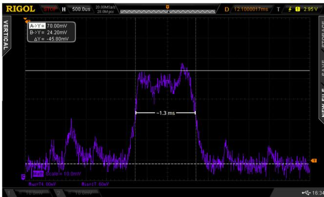
Fig. 17: Oscilloscope screenshot from a packet transmission on the 3 advertising channels.
