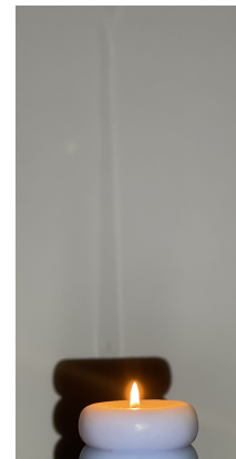
Figure 18: Shadow graph of a candle showing the hot air plume rising from the flame
