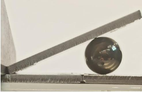
Figure 51: Friction test set-up steel ball on aluminium plate
