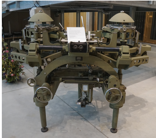
Figure 5: Picture of stereoscope in Langezijds at University of Twente, with two lenses visible.
