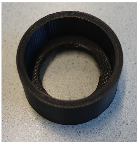
Figure 32: Test print of a tube (approximately 49 mm in diameter) to see if it could fit around the microscopic lens, in this case it did not.
