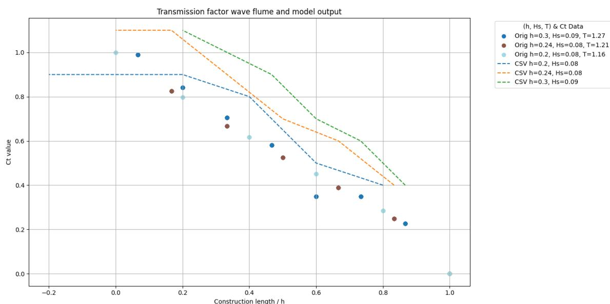
Figure 29: A comparison of the transmission factor predicted by the model and the transmission factors determined in the wave flume experiment. This is done for different water depths, wave heights, and wave periods.
