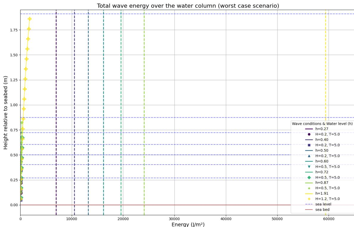
*Figure 38: Overview of the critical wave energy, related to the critical bed shear stress for sediment deposition, together with the simulated cumulative total wave energy*
