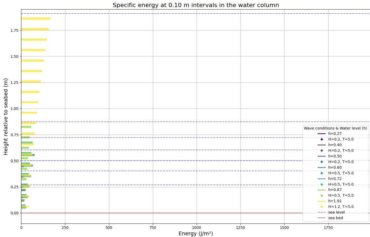
Figure 18: Wave energy corresponding to specific points in the water column. The x-axis shows the wave energy in  $J/m^2$ , and the y-axis shows the height relative to the seabed. Each bar represents the depth-specific wave energy at that height relative to the seabed.
