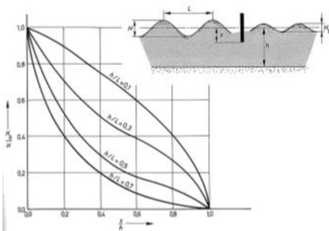
Figure 15: Graph Nortier & de Koning (1996) showing the transmission factor corresponding to different construction height water depth ratios for different wave steepnesses
