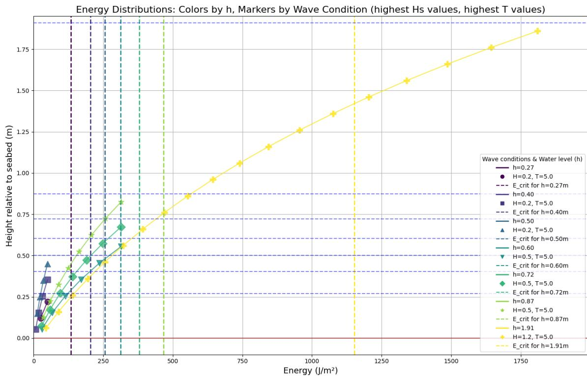
Figure 28: Total cumulative wave energy at 0.10 meter intervals in the water column for each water depth within the determined tidal range, AND the corresponding critical wave energy. The x-axis shows the wave energy in  $J/m^2$ , and the y-axis shows the height relative to the seabed. Each solid line represents the depth-specific wave energy at that height
