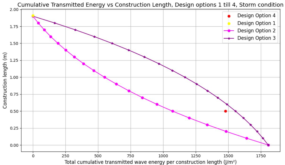
Figure 25: Overview of the total cumulative transmitted energy ( $J/m^2$ ) (on the x-axis) generated by different construction heights (m) (on the y-axis) per Design Option for the storm condition.
