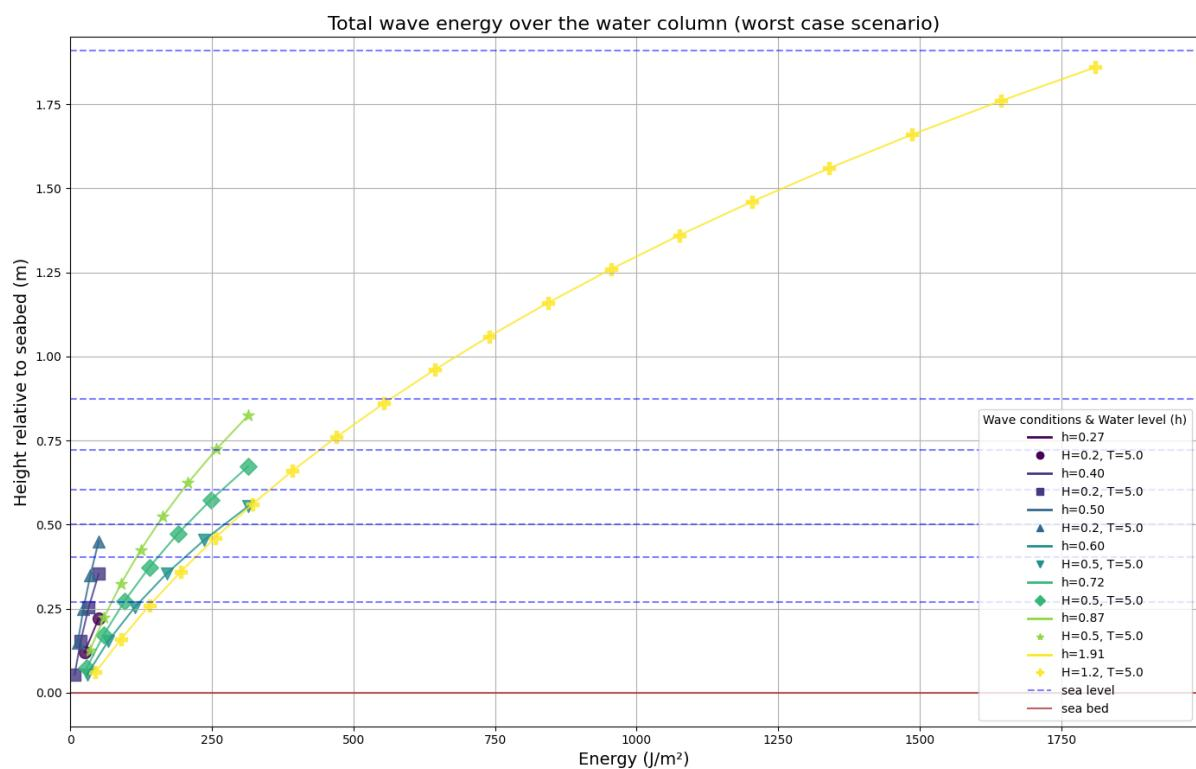
Figure 17: The graph shows the cumulative total wave energy distribution over the water column, with the wave energy in  $\text{J}/\text{m}^2$  on the x-axis. On the y-axis, the height relative to the seabed is shown. Each marker point represents the total wave energy at that height relative to the seabed.
