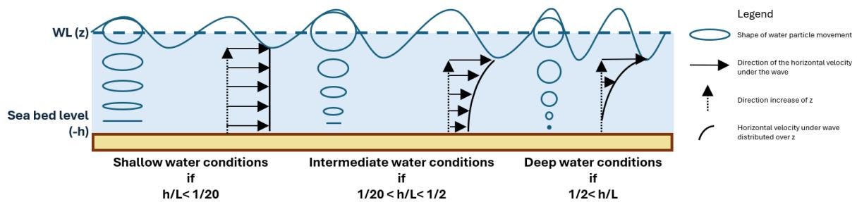
Figure 6: Orbital particle movements and velocities under shallow, intermediate, and deep water conditions
