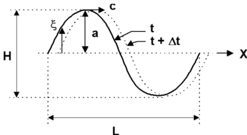
Figure 5: sinusoidal wave according to linear wave theory with wave height  $H$  [m], wave length  $L$  [m], phase velocity denoted as  $c$  in the figure but notated as  $c_w$  in the equations (Van Der Werf, 2024)
