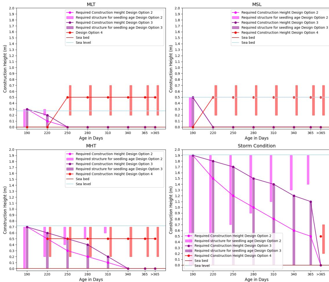
Figure 34: The required construction heights (plotted as lines) and corresponding positioning (plotted as bars) of Design Options 2, 3, and 4 are shown for each water level (MLT, MSL, MHT, and the storm condition).
