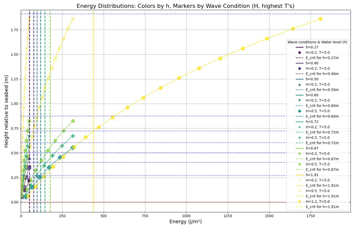
Figure 7: Cumulative total wave energy distribution for all water levels, wave heights, and wave periods together with the critical wave energy for mangrove seedlings of an age of 250 days
