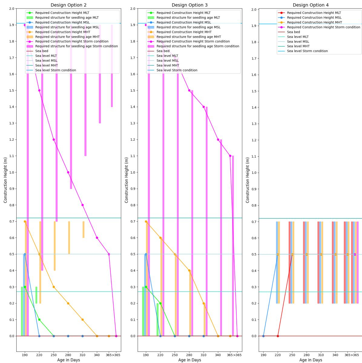
Figure 35: The required construction heights (plotted as lines) and corresponding positioning (plotted as bars) of Design Options 2, 3, and 4. Per design Option the different water depth scenarios are simulated.
