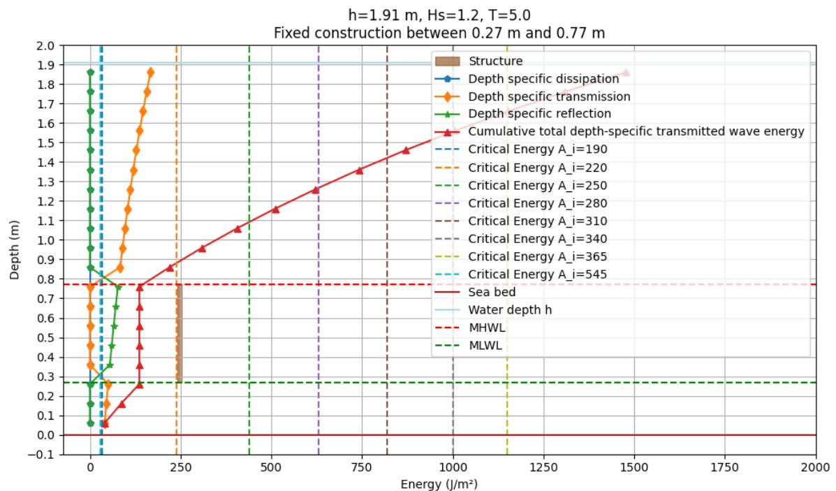
Figure 32: Model output of the simulation of design option 4 under storm conditions
