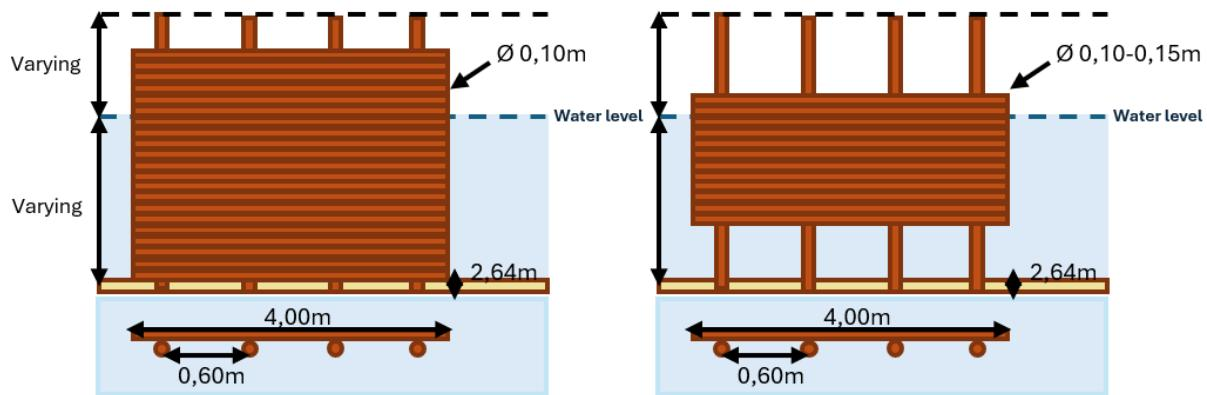
Figure 12: Sketch of permeable structure that will be implemented into the analytical (wave) model
