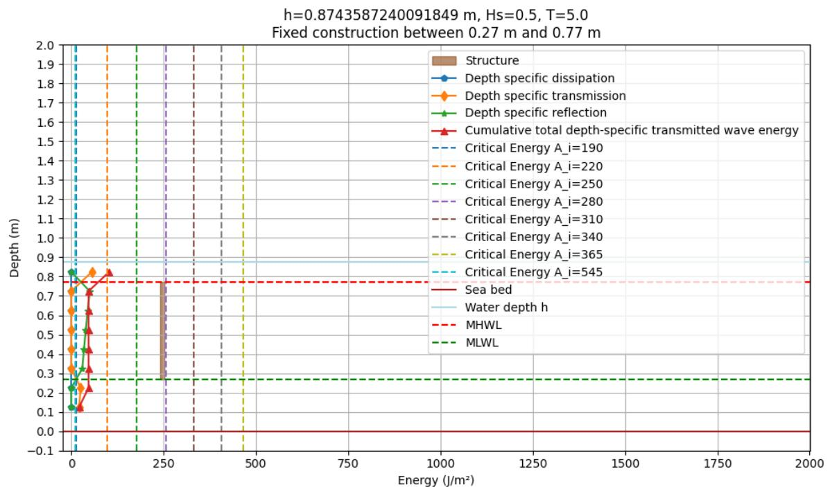
Figure 31: Model output of the simulation of design option 4 under SHT conditions
