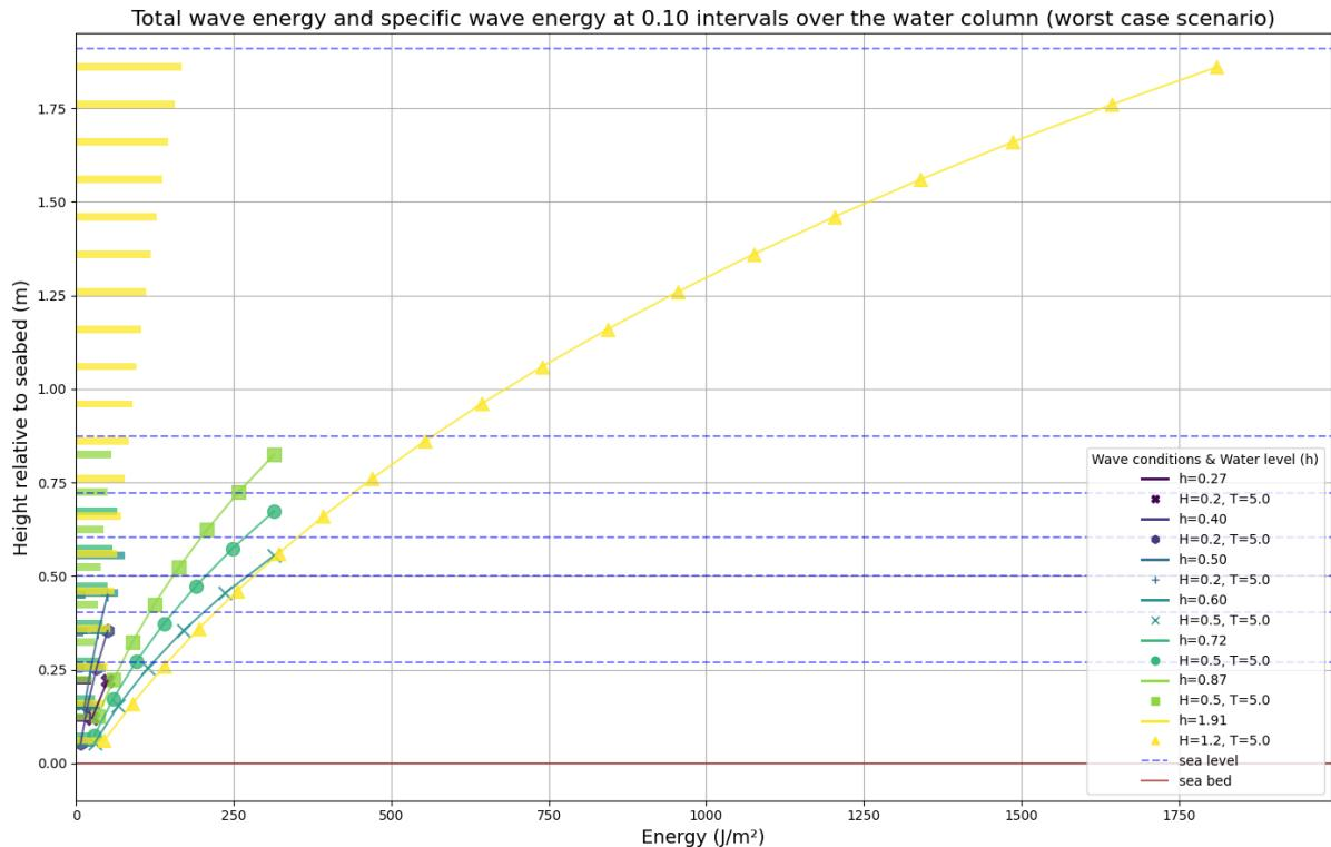
**Figure 19:** Combination of the representation of the wave energy corresponding to specific points in the water column and the cumulative total wave energy at 0.10-meter intervals in the water column. The x-axis shows the wave energy in  $J/m^2$ , and the y-axis shows the height relative to the seabed. Each bar represents the depth-specific wave energy at that height relative to the seabed. The lines represent the cumulative total wave energy distribution.
