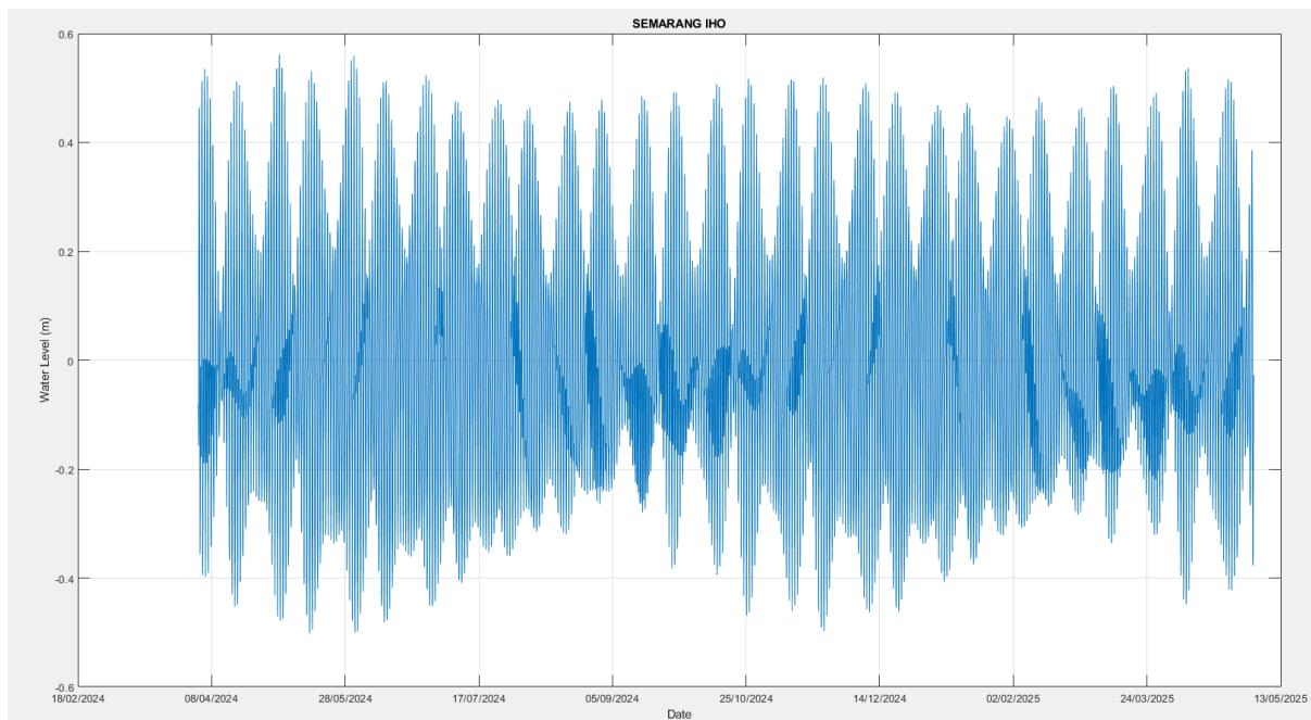
Figure 1:: Tidal spectrum based on IHO data Semarang between 4-10-2024 and 4-10-2025
