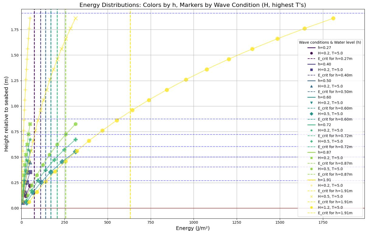
*Figure 8: Cumulative total wave energy distribution for all water levels, wave heights, and wave periods together with the critical wave energy for mangrove seedlings of an age of 280 days.*
