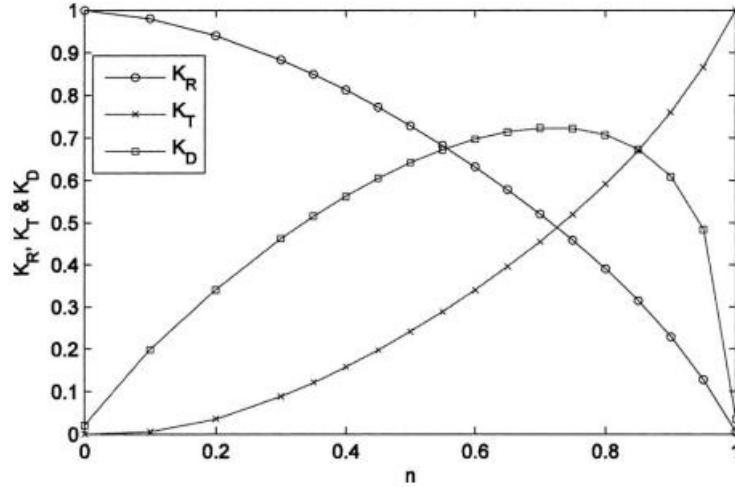
Figure 36: Different transmission, reflection and dissipation coefficients under different porosities (Lin & Karunaratna, 2007)
