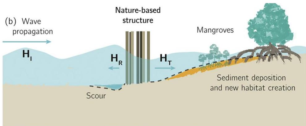
Figure 4: Wave attenuation and sediment deposition in case of a permeable dam (Gijón Mancheño et al., 2021a)
