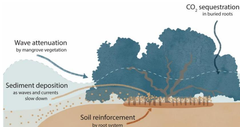
Figure 1 Sediment deposition, wave attenuation, and soil reinforcement by mangroves (Gijón Mancheño, 2022)
