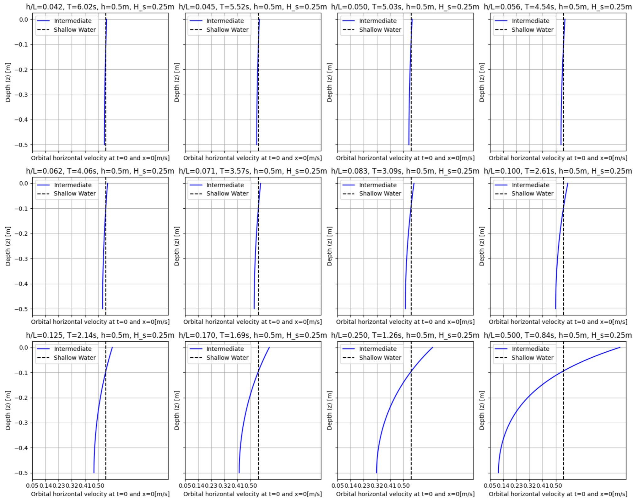
Figure 4: Orbital horizontal velocities for different  $h/L$  fractions
