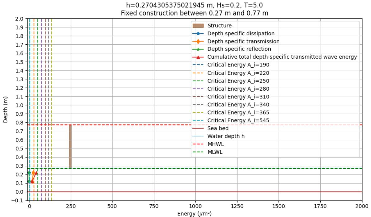
Figure 26: Model output of the simulation of design option 4 under MLT conditions
