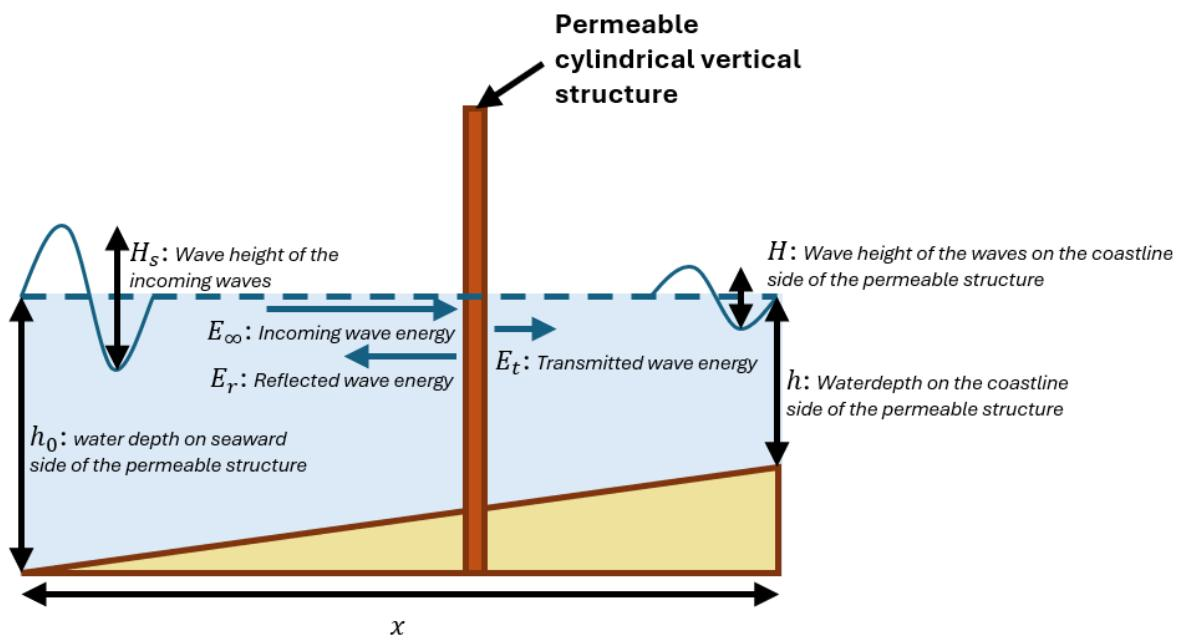
Figure 10: The influence of a permeable structure on wave propagation
