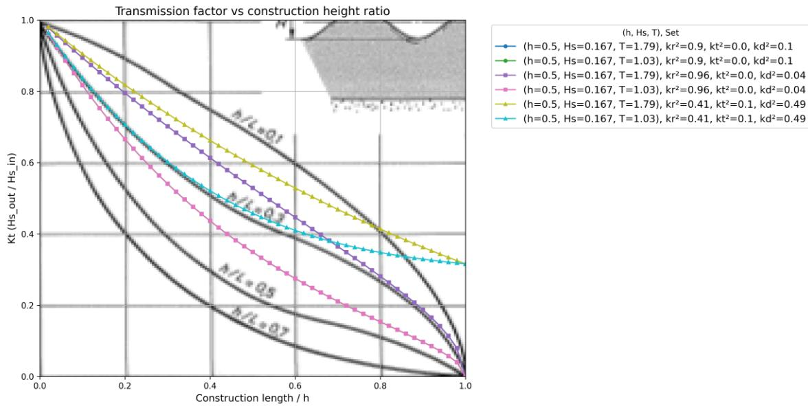
Figure 37: Comparison of model results under applied transmission, reflection, and dissipation coefficients to Nortier & de Koning (1996)
