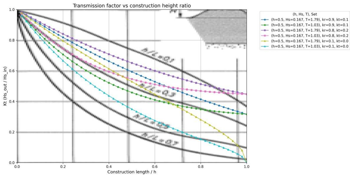
Figure 33: Comparison of Nortier & de Koning (1996) and model results. The graph of Nortier & de Koning (1996) shows the construction height- to water depth - ratio for wave steepnesses of 0.1, 0.30 , 0.5 and 0.7.
