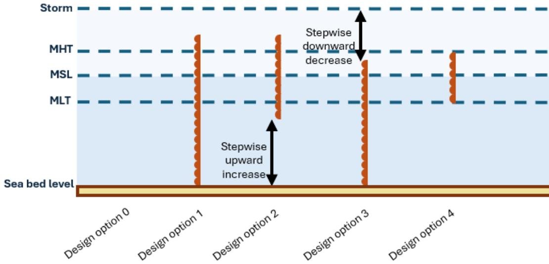
Figure 14: Sketch of the different design options for the permeable structures that will be implemented into the analytical Python model
