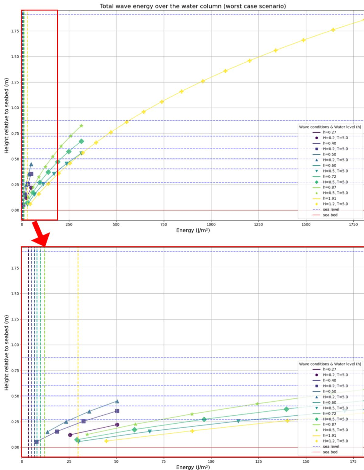
Figure 39: Overview of the critical wave energy, related to the critical bed shear stress for erosion, together with the simulated cumulative total wave energy
