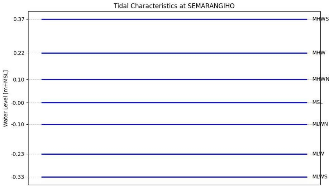
Figuur 2: Tidal range based on IHO data Semarang between 4-10-2024 and 4-10-2025. Relative to MSL.
