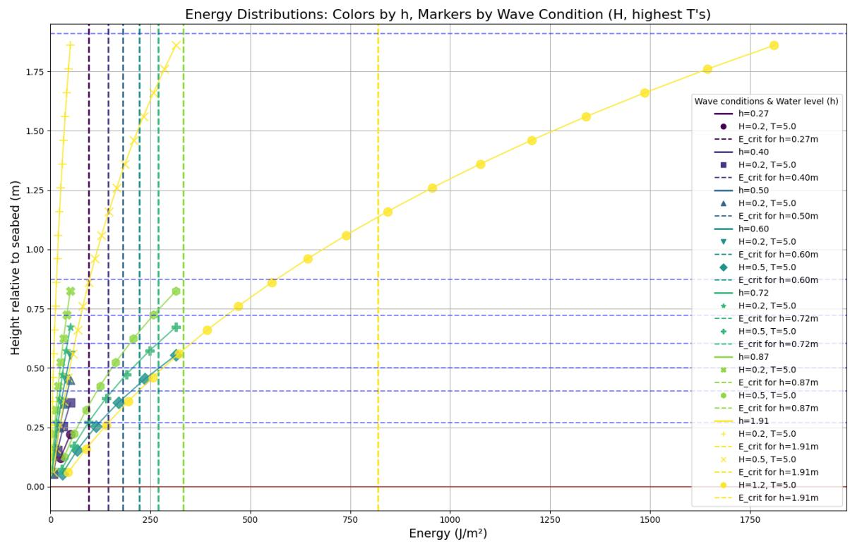
Figure 9: Cumulative total wave energy distribution for all water levels, wave heights, and wave periods together with the critical wave energy for mangrove seedlings of an age of 310 days
