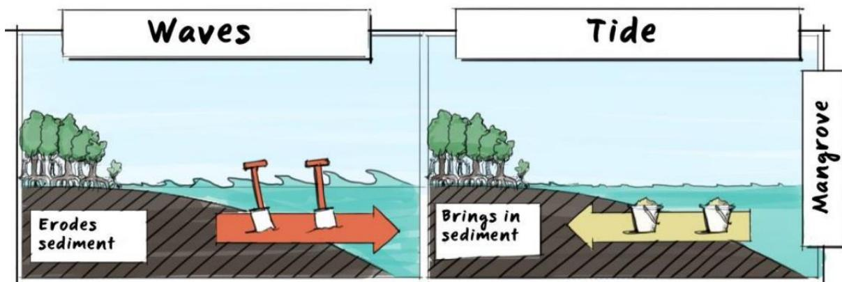
Figure 8: Visualisation of the impact of waves and tide on sediment transport (H. Winterwerp et al., 2014)
