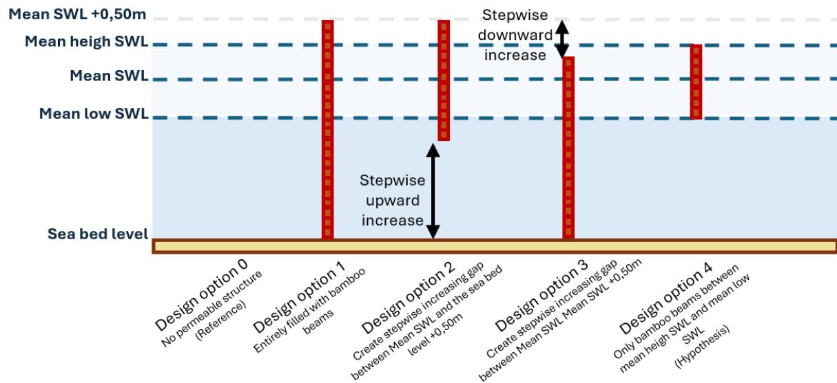
An optimization will be conducted, to find the design that causes a certain transmitted wave height while using the least amount of material.
