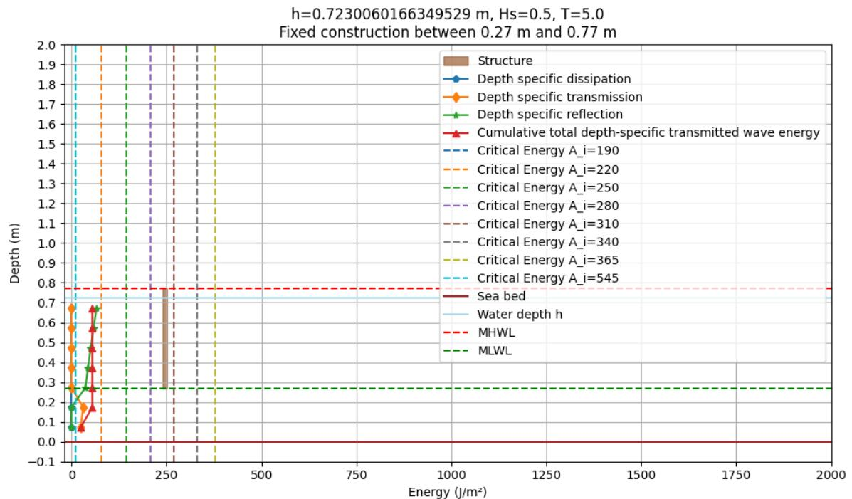
Figure 30: Model output of the simulation of design option 4 under MHT conditions
