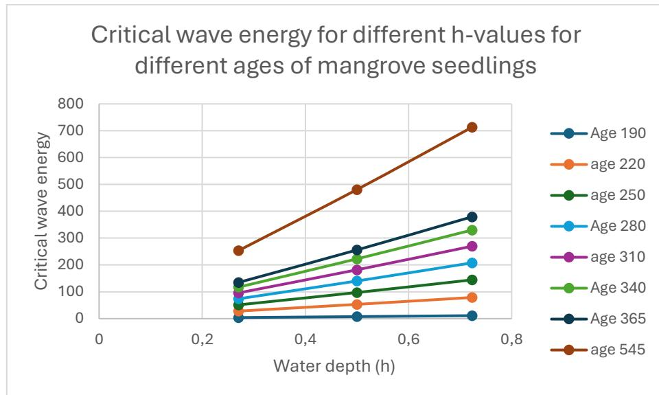
Figure 27: Overview of critical wave energy for different  $h$ -values for different ages of mangrove seedlings. The y-axis shows the critical wave energy in  $J/m^2$ , and the x-axis shows the water depth ( $h$ ) in meters. Each seedling age has its color.
