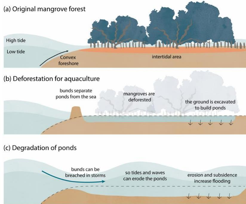
Figure 3: How aquaculture deforests mangroves and causes erosion (Gijón Mancheño, 2022)
