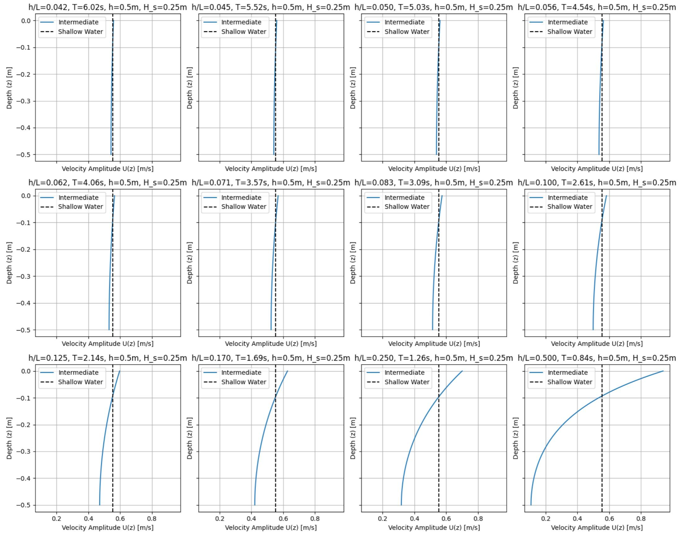
Figure 5: Velocity amplitudes for different  $h/L$  fractions
