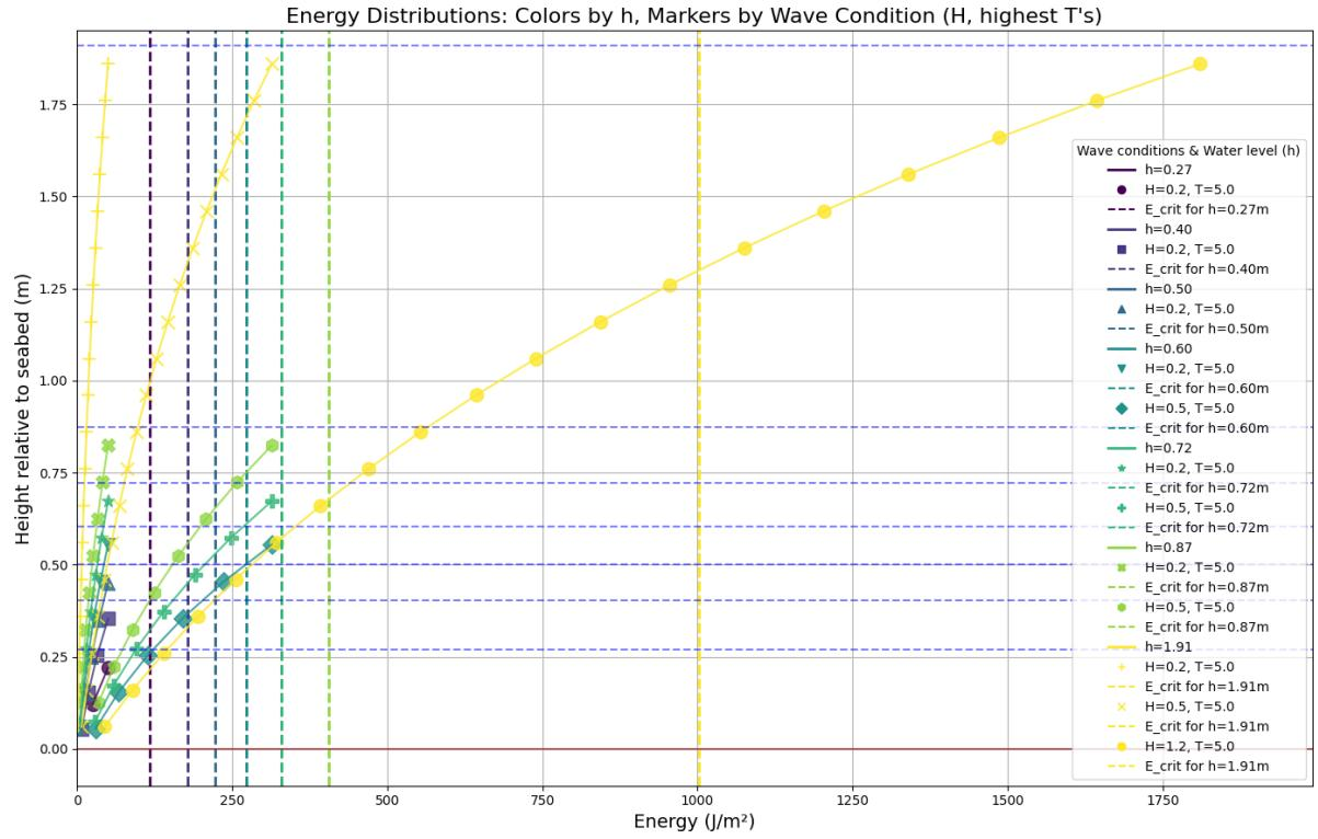
Figure 10: Cumulative total wave energy distribution for all water levels, wave heights, and wave periods together with the critical wave energy for mangrove seedlings of an age of 340 days
