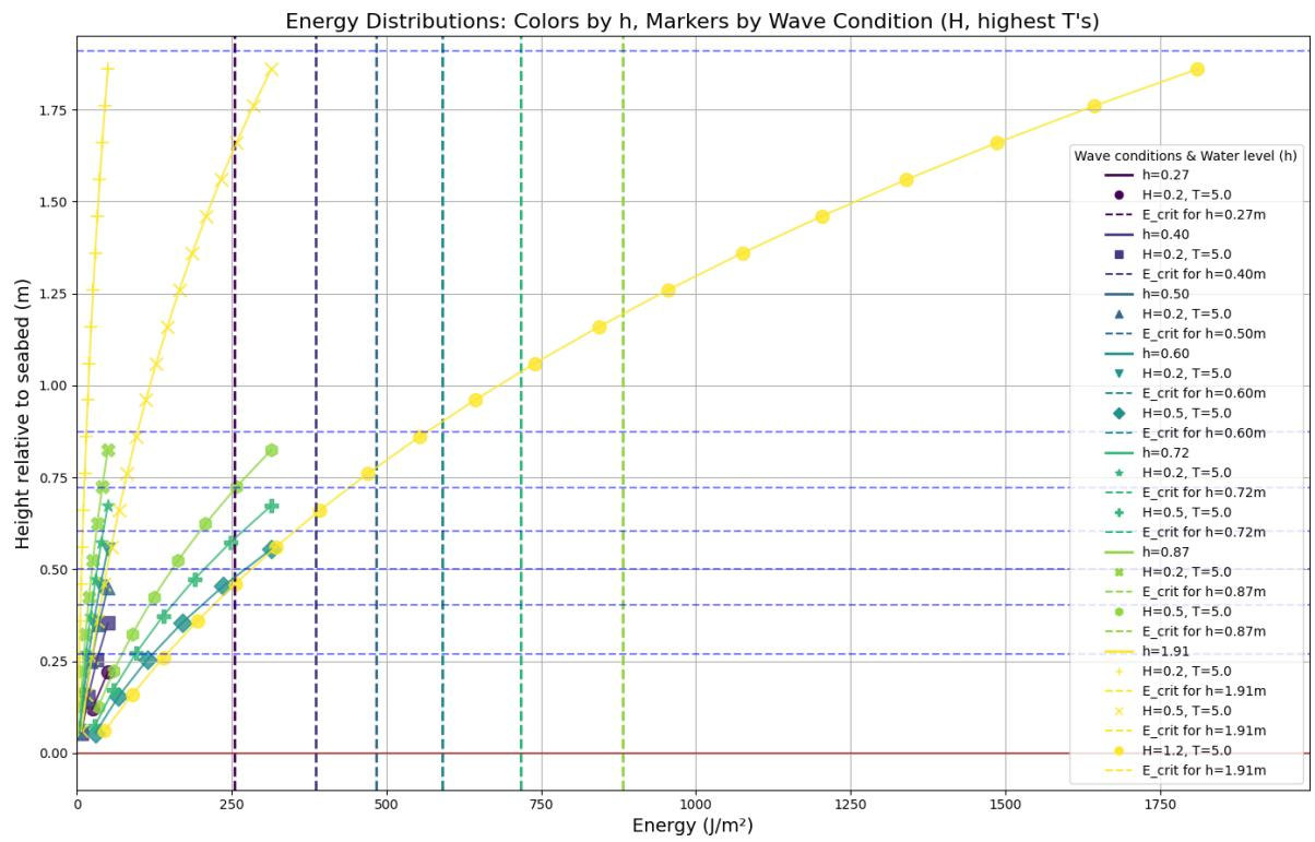
Figure 11: Cumulative total wave energy distribution for all water levels, wave heights, and wave periods together with the critical wave energy for mangrove seedlings of an age of 545 days.
