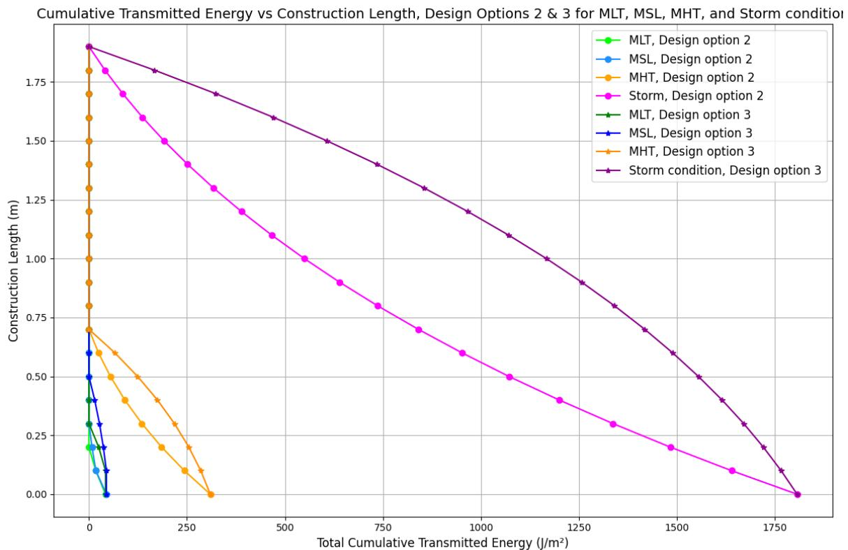
Figure 26: Overview of the total cumulative transmitted energy ( $J/m^2$ ) (on the x-axis) generated by different construction heights (m) (on the y-axis) for Design Options 2 and 3 for all water conditions.
