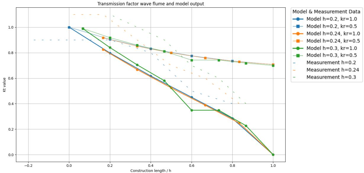
Figure 31: Comparison of model output and wave flume experiment data
