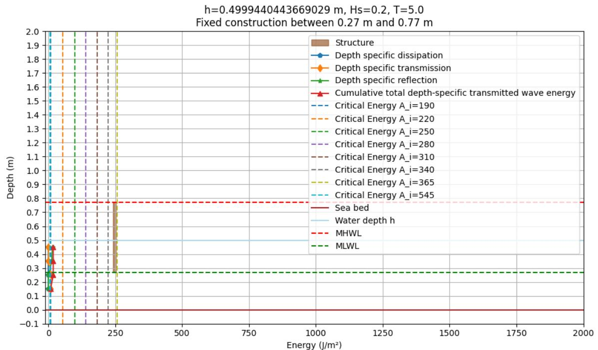
Figure 28: Model output of the simulation of design option 4 under MSL conditions
