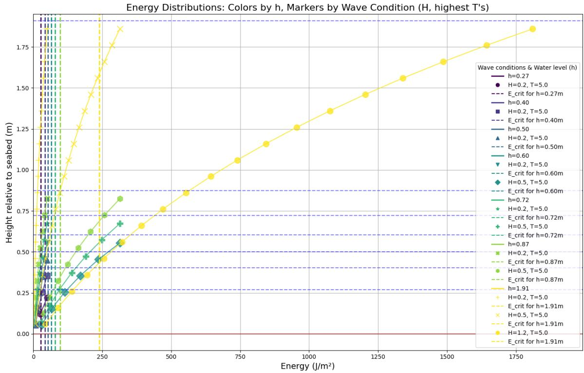
Figure 6: Cumulative total wave energy distribution for all water levels, wave heights, and wave periods together with the critical wave energy for mangrove seedlings of an age of 220 days
