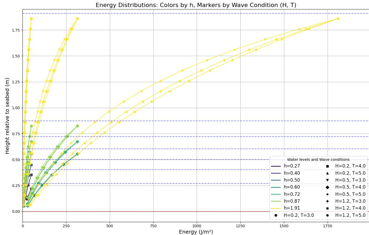
Figure 6: Cumulative total wave energy distribution for all water levels , wave heights, and wave periods
