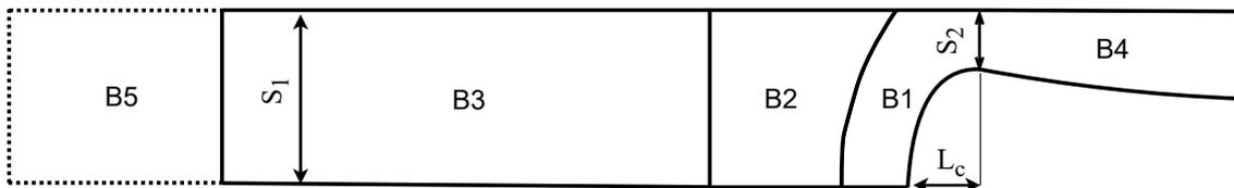
FIGURE 2.4: Schematic of multi-block numerical domain with  $S_1/S_2 = 3$
