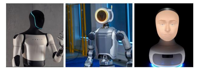
*Note*. From left to right: Tesla's Optimus Gen 2, the Atlas robot from Boston Dynamics, and the Furhat robot from Furhat Robotics. Of the robots shown, only Furhat includes an integrated gaze system.
