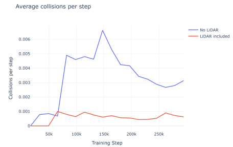
Fig. 1. Average collisions per step during the training with LiDAR and without. The X-axis represents training time steps, whereas Y-axis describes the number of collisions per step based on the rollout average. Number of collisions per rollout can be roughly calculated by multiplying graph's value by N\_Envs \times N\_Steps .
