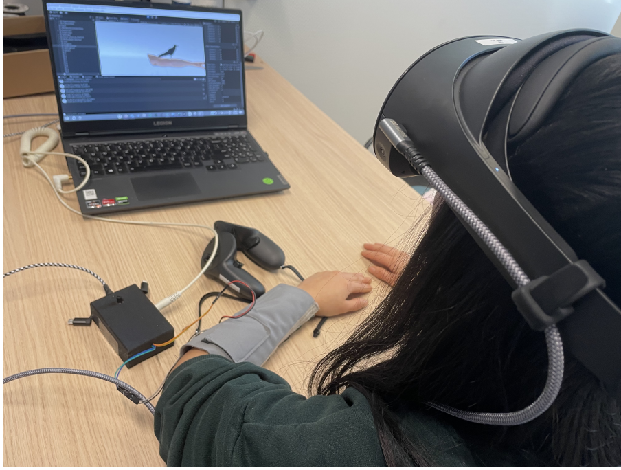
FIGURE 6: Set up of de Zwaan's [6] VR visual and vibrotactile sleeve
