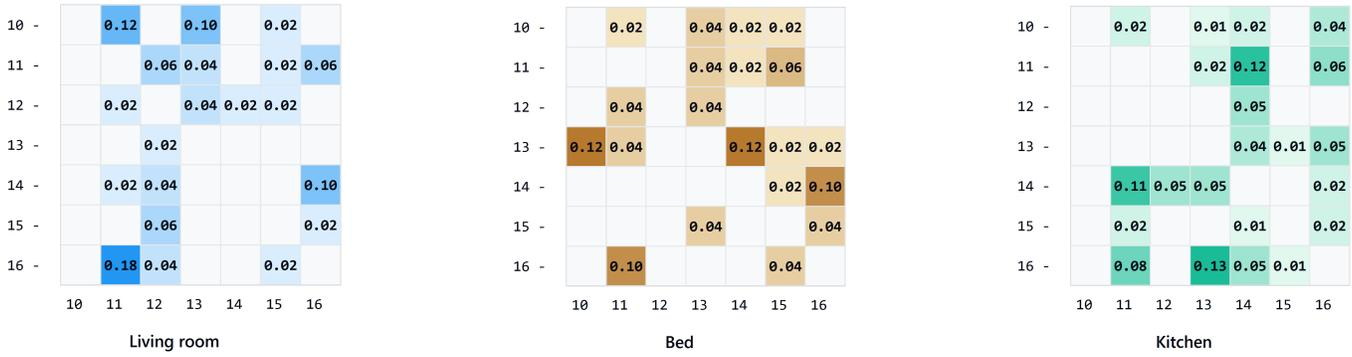
Fig. 5. Node distribution for the different rooms after CNN-based initialization. Entries represent how often a receiver (row) was paired with a transmitter (column).
