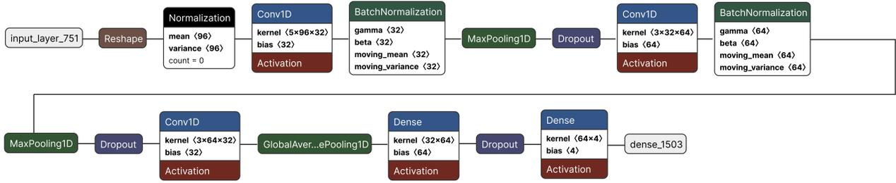
Fig. 3. Architecture of the Convolutional Neural Network (CNN) used in this study. The model consists of multiple convolutional and pooling layers for feature extraction, followed by fully connected layers for classification. Each layer is annotated with its output shape and activation function.
