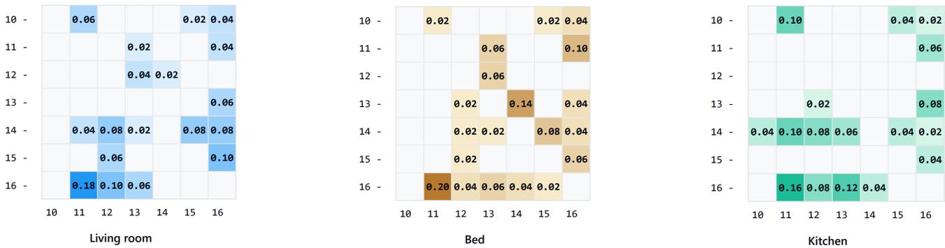
Fig. 7. Node distribution for the different rooms after CNN based initialization phase implementing fluctuation-based exclusion, where the entry represents how many times a receiver (row) was paired with a transmitter (column).
