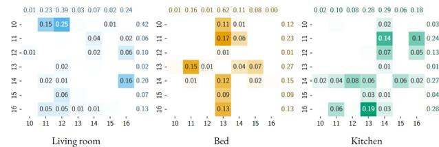
Fig. 2. Node distribution for the different rooms after the initialization phase where the entry represents how many times a receiver (row) was paired with a transmitter (column) [2].
