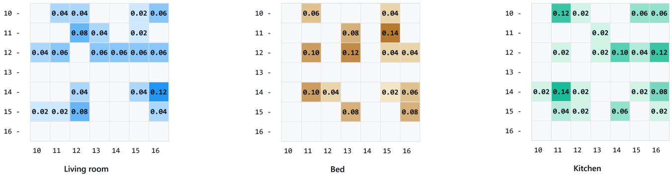
Fig. 6. Node distribution for the different rooms after CNN based initialization phase implementing filtering by RSSI, where the entry represents how many times a receiver (row) was paired with a transmitter (column).
