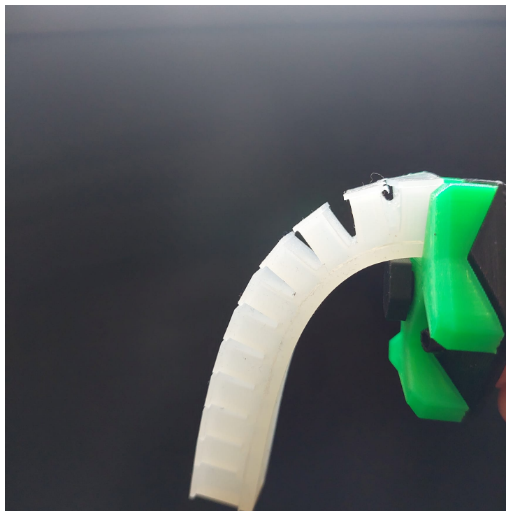
Figure 5.2: Amount of Bending in the first finger prototype
