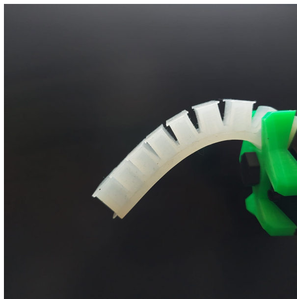
Figure 5.4: Amount of Bending in the second finger prototype
