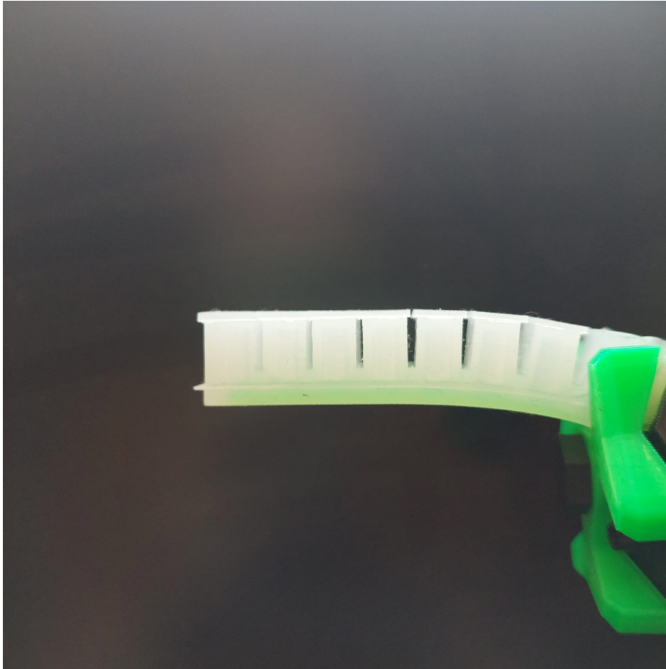
Figure 6.4: Amount of Bending in the final finger prototype
