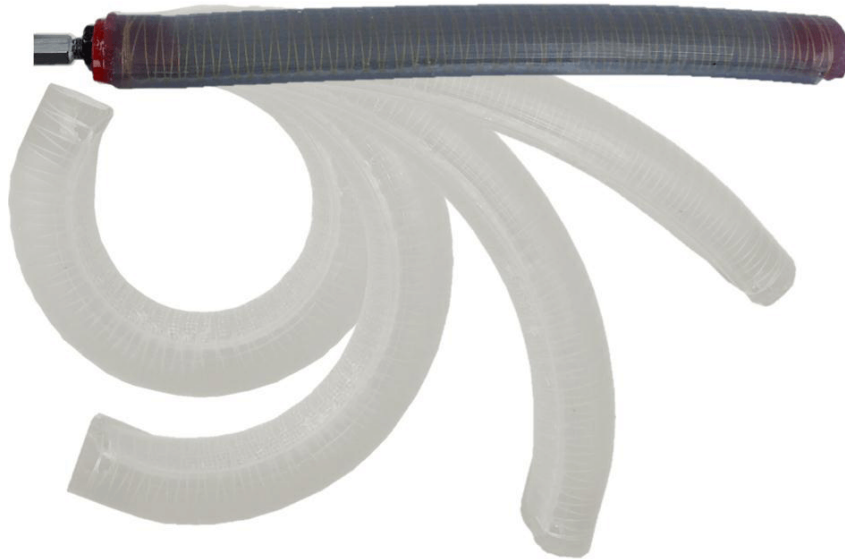
Figure 2.4: Fiber-Reinforced Actuator Bending [17].
