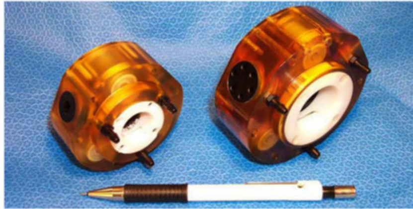
Figure 2.7: Two Stepper Motor Prototypes of The PneuStep [18].
