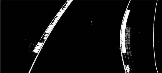
Fig. 4. Found track boundaries (red dots) displayed on the binary image for visual confirmation.
