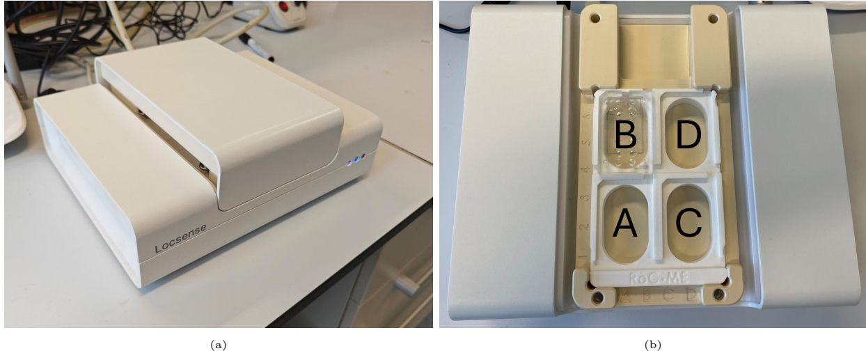
Figure 6: The Locsense Artemis ST system. (a) The Artemis from the outside with the base and the lid. (b) The holder in the base of the Artemis system for four chips with the possible positions A, B, C and D.
