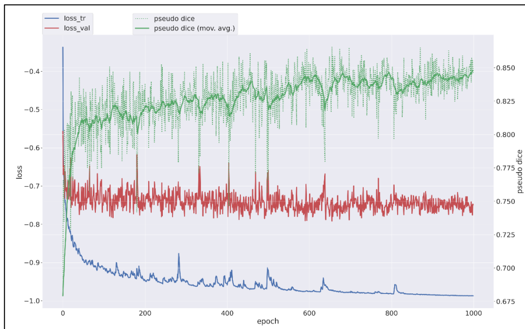
Figure 1.7: Training log of learning curves of the transverse 5-FCV network. The training loss is presented in blue and the validation loss in red.
