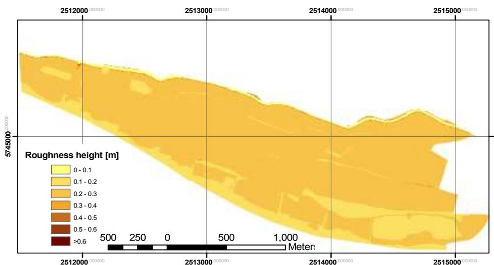
Figure 5-19: Roughness distribution over the floodplain, grassland coverage (see section 3.2), HHQ of 1995
