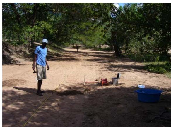
*Figure 18: Resistivity test in the alluvial aquifer*
