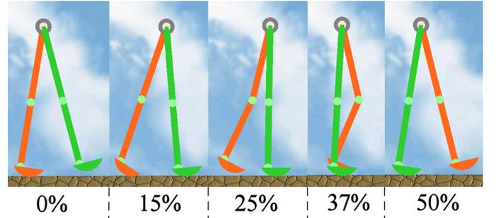
Fig. 10. Composure of robot at percentages of stride time
