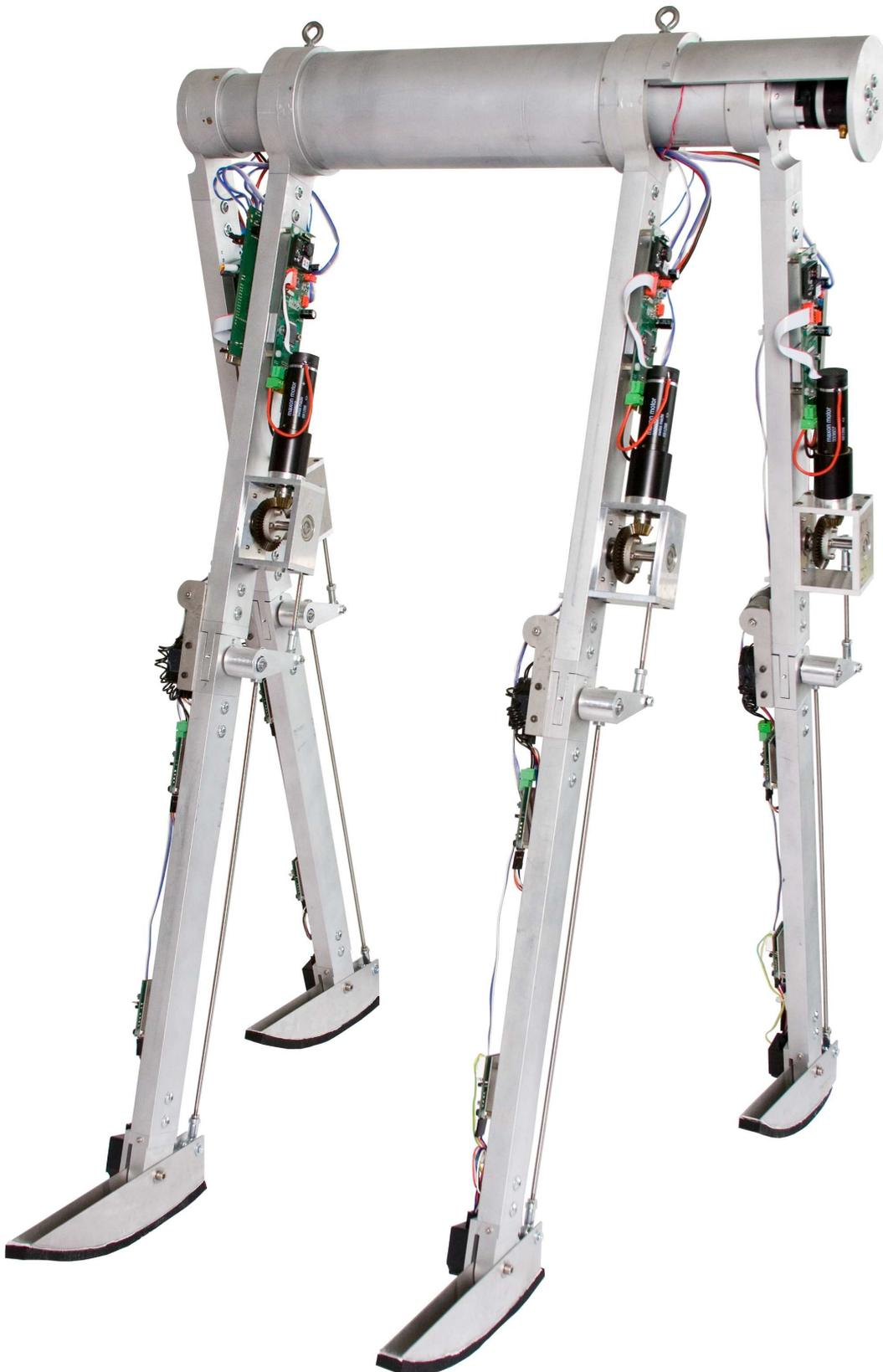
Fig. 5. Dribbel with added feet and ankle actuation system (Photo taken by M.H. Schwirtz)
