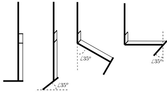
Fig. 6. Sketch of the transmission and its three extreme poses
