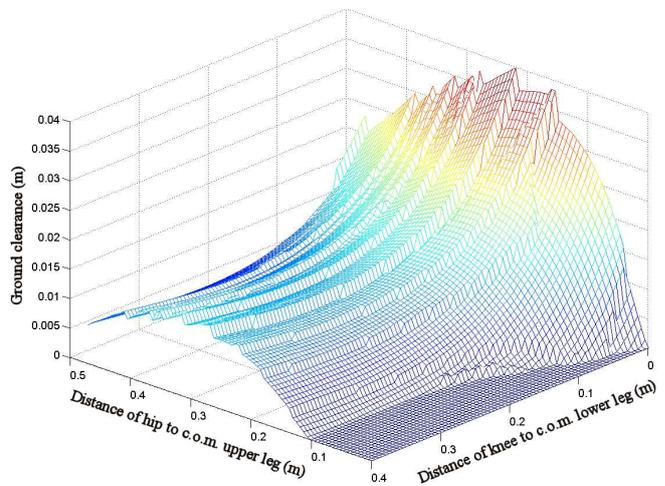
Fig. 5. Ground clearance as function of location of limb c.o.m.
