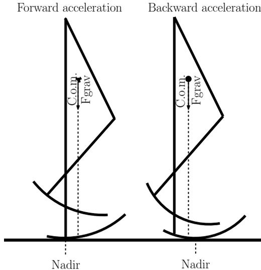
Fig. 8. Rolling of stance leg due to location of c.o.m.
