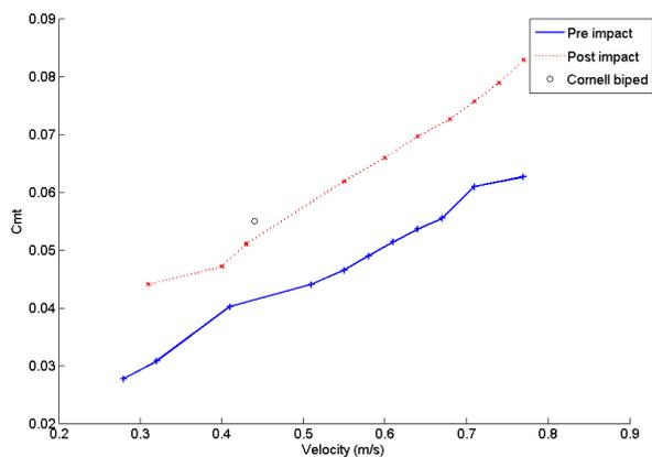
Fig. 11. Specific mechanical cost of transport as function of velocity
