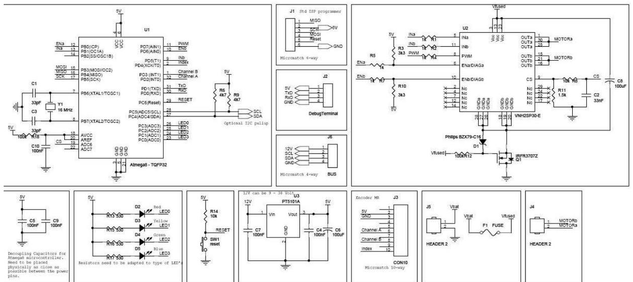
by hardware. To remedy this the PWM and INa signals switch I/O ports on the microcontroller. In the physical board the switch between the tracks is made by placing R1 and R4 in an upright position and reconnecting their output to the proper track.
