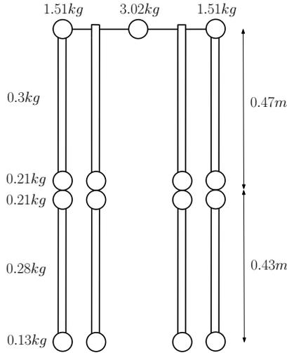
Fig. 2. Mass distribution in current configuration
