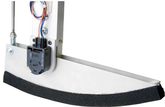
Fig. 4. Foot and ankle joint
