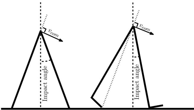
Fig. 3. Effects of a push off with the foot on the impact angle and velocity
