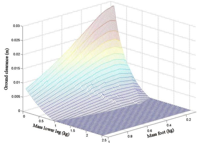
Fig. 4. Ground clearance as function of mass distribution
