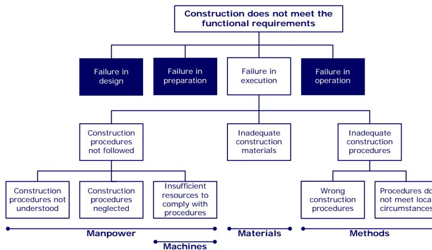
Figure 5: Failure tree for analysing the possibilities of failure in Indian road construction processes
