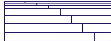
Figure 12: Joints within several layers
