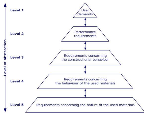
The requirements of the pyramid are being transferred from a high level towards lower levels of abstraction. For example: A user demands a safe and comfort ride. These demands are translated into performance requirements like a level and rough surface which reduces noise. These requirements subsequently create requirements for the entire pavement construction, as well as to the raw materials that are used. Figure 10 visualizes the different levels of abstraction.
