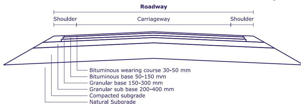
**Figure 9: Typical flexible pavement components (MORTH; 2001)**
