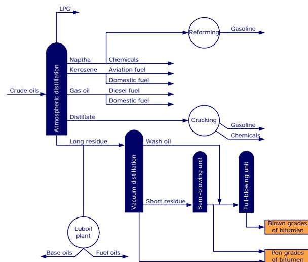
**Figure 18: Distillation process of crude oil (Read&Whiteoak; 2003)**
