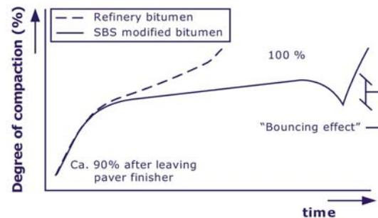
**Figure 19: Schematic representation of compaction behaviour of asphalt mix built out of conventional and modified bitumen**
