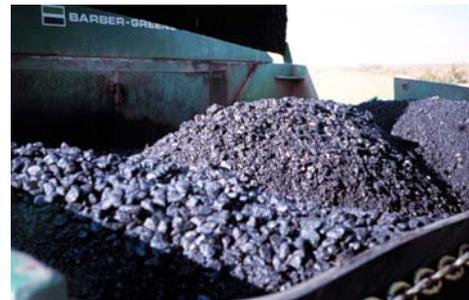
**Figure 14: Segregation in receiving hopper of an asphalt paver finisher**
