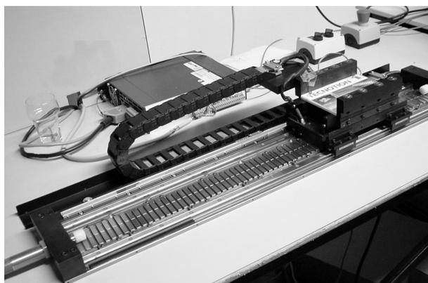
Figure 4.1: The Tecnotion linear motor
