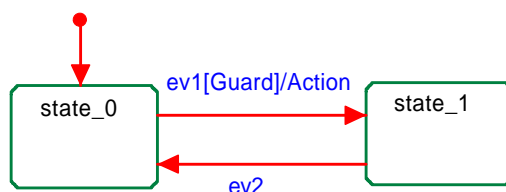
Figure 26 : Statechart diagram with transition, guard and action
