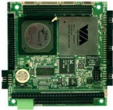
Figure 51: Seco M570-BAB Via Eden ESP 600 MHz
