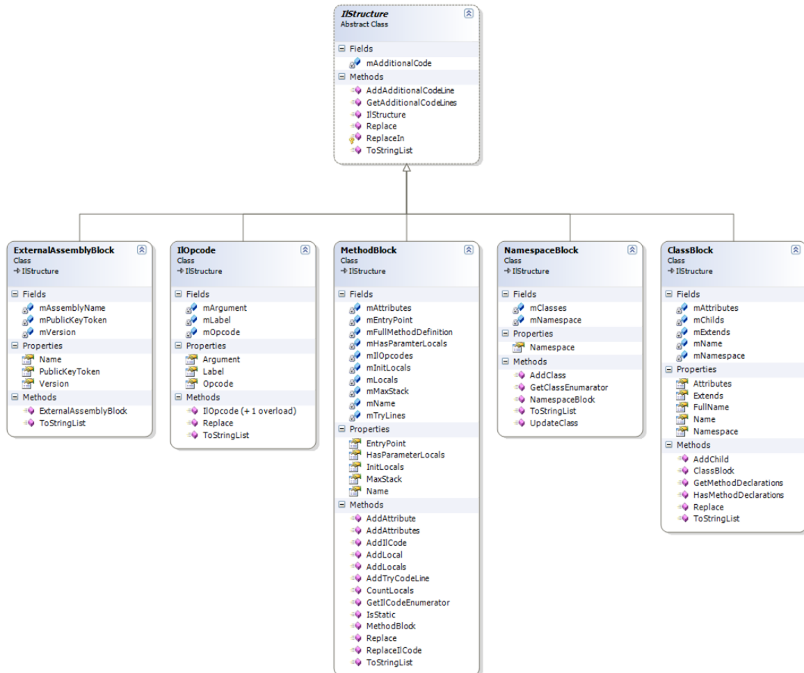
Figure D.4: Class diagram internal IL representation, the ILStructure .
