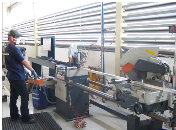
Fig.3: Semi automatic cutting of aluminium profiles
