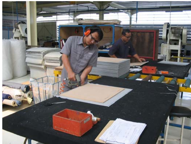
Fig.9: Producing a panel of a workstation
