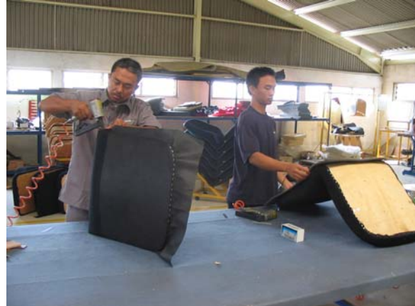
Fig.8: Attaching the fabric to the seat
