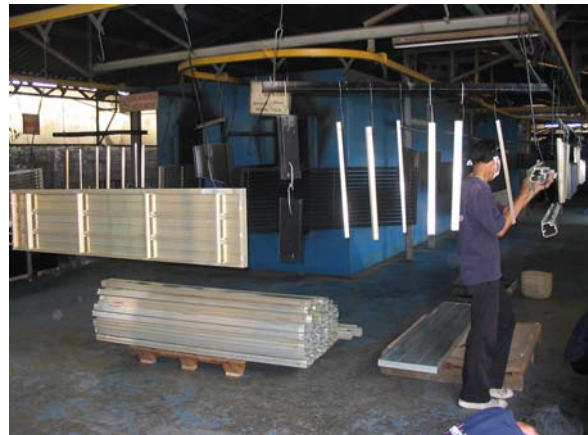
Fig.5: Applying powder coating
