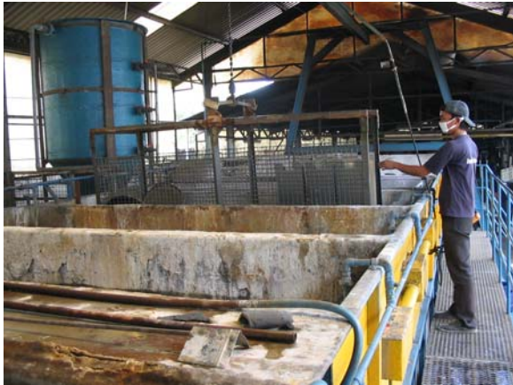
Fig.4: Chemical baths for cleaning and preprocessing metal parts
