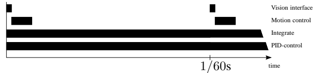
Fig. 2. Task execution scheme — There are three real-time tasks that run simultaneously: the motion control algorithm at low frequency (60 Hz. or higher), setpoint generation through integration (1 kHz. or higher) and closed loop actuator control and interfacing (also 1 kHz. or higher). Interfacing the vision algorithm is not a real-time task.
