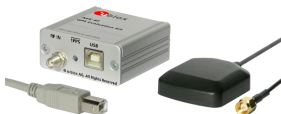
Figure 5.1: u-Blox AEK-4H evaluation receiver package with external antenna
