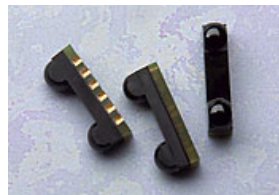
Figure 4.3: Avago IrDA transceiver (size: 1.60 x 7.00 x 2.73 mm)
