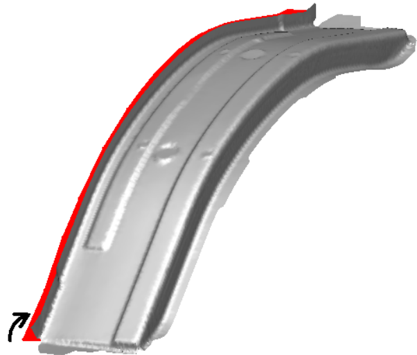
Fig. 5.1 the OP50 forming stage: bending the flange
