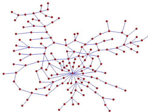
Figure 2: Example of a network. This is a graph representation of the optical fibre network from the Spanish province Teruel (however not a geographical representation).
