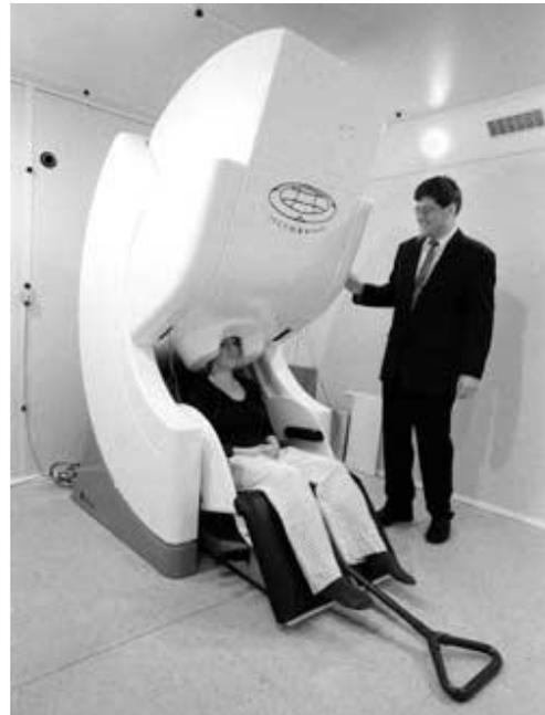
Figure 5 - An MEG machine, located at the Martinos Center for Biomedical Imaging at Massachusetts General Hospital-East.
