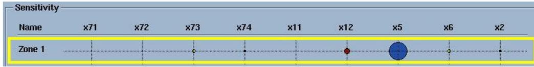
(a) BHF =  $3.51 \times 10^6$  N, response Failure
