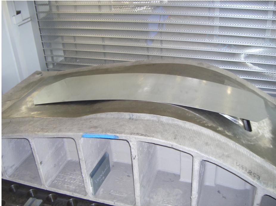
Figure E.3: Position of the blank on the die
