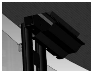
Figure 62 - Fixation of the front leg
