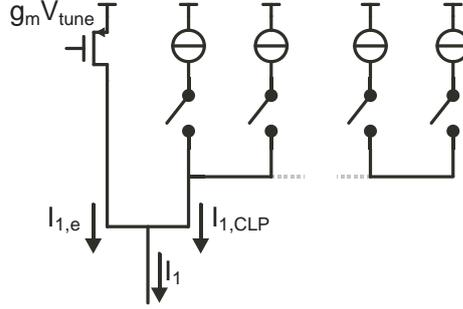
Figure 5.12: Semi-discrete current source  $I_1$
