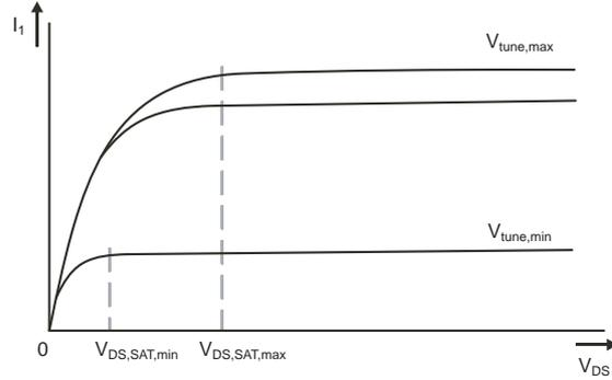
Figure 5.11:  $V_{DS} \neq V_{DS,SAT}$  due to change in  $V_{tune}$
