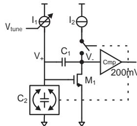
Figure 3.1: Switched capacitor relaxation oscillator
