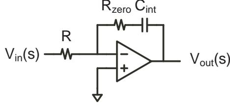
Figure 6.3: Integrator with a zero added
