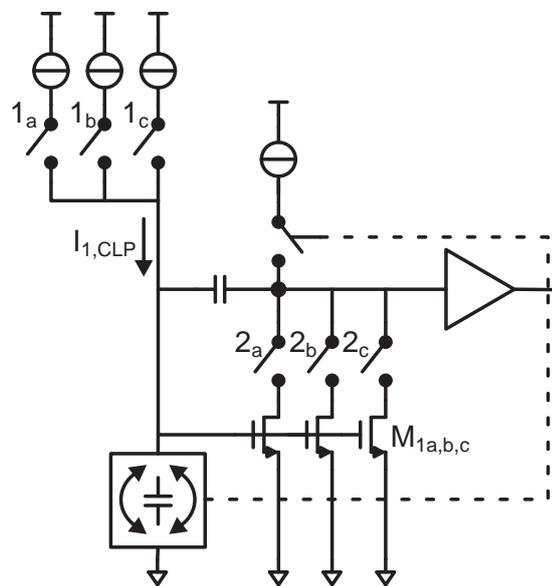
Figure 5.25: Constant  $\Delta V_2 = 2 \cdot V_{GS, M_1}$  during RL-Phase
