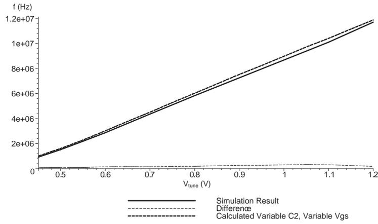
Figure 4.9: Frequency calculation with  $C_{GS}$  taken into account
