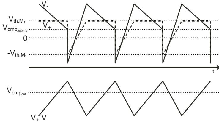
Figure 3.2: Oscillator signals
