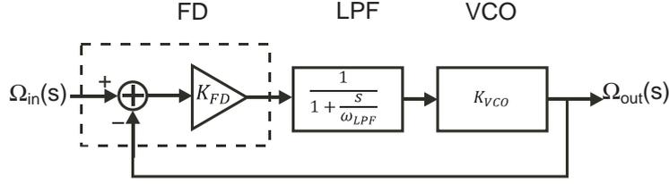
Figure 1.7: Frequency-locked loop (FLL)
