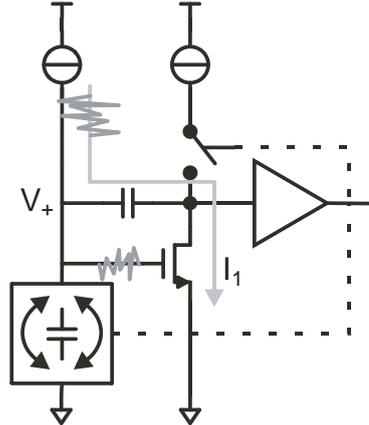
Figure 5.9: Noise in  $I_1$  results in a variable charge packet
