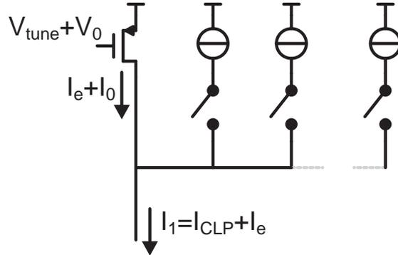
Figure 5.37: Alternative for presetting the integrator
