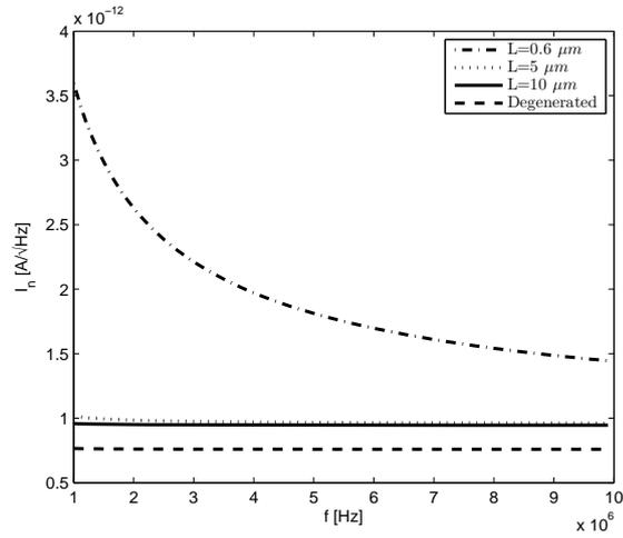
Figure 5.16:  $I_1$  output referred noise results for non-degenerated PMOS transistors
