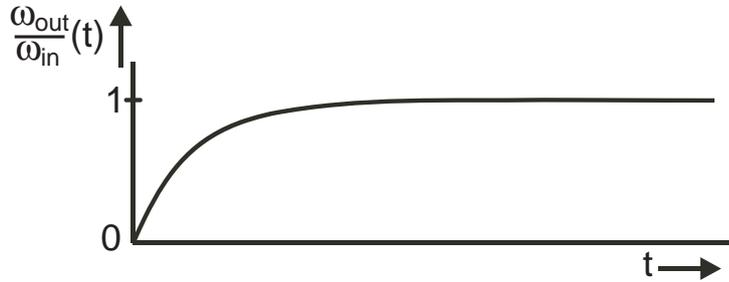
Figure 1.8: Impression of Frequency-Locked Loop in time domain
