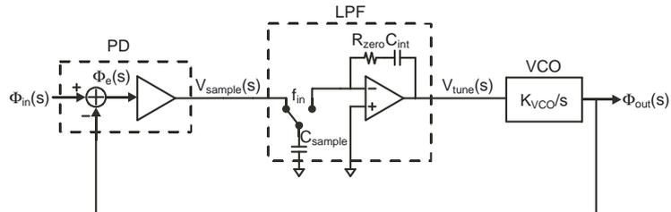
Figure 6.1: Graphical model of the PLL
