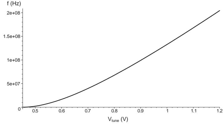
Figure 4.2: Frequency calculation with non-degenerated current source
