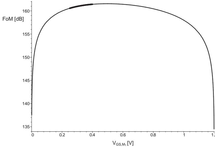
Figure 5.26: FoM calculation of the original oscillator
