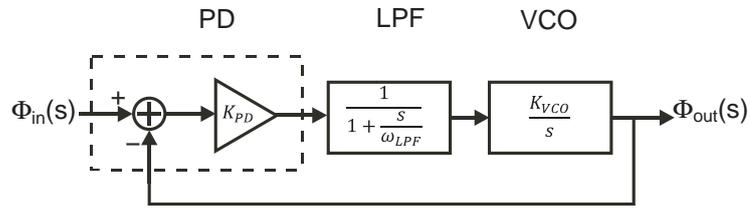
Figure 1.3: General phase detector with gain  $K_{PD}$
