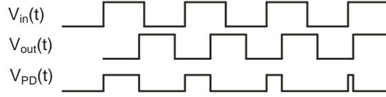
Figure 1.2: Output signal of a simple phase detector
