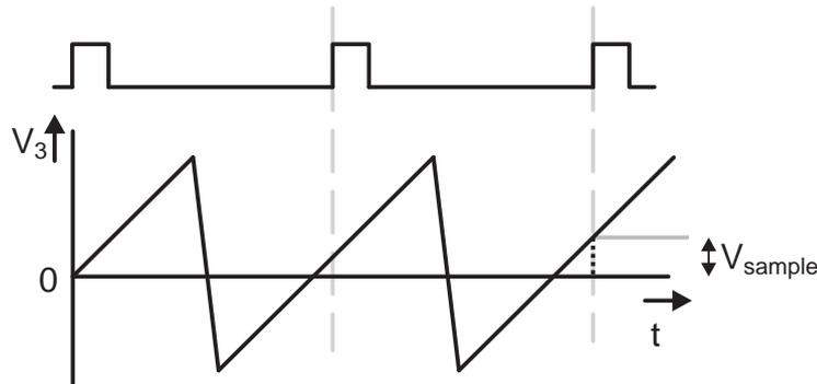
Figure 5.29: Acquisition of a representation of  $\phi_e$  through  $V_{sample}$
