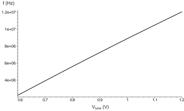
Figure 4.3: Frequency calculation with degenerated current source
