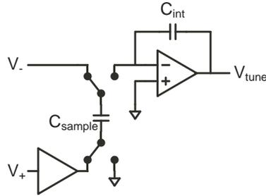
Figure 5.32: Differential to single-ended integrator
