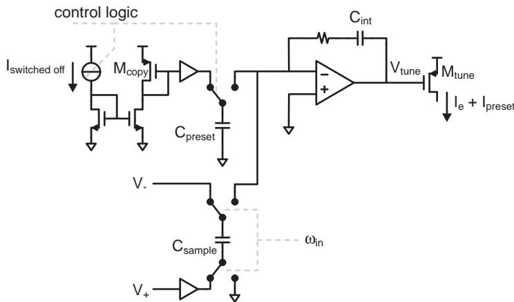
Figure 5.36: Presetting the integrator
