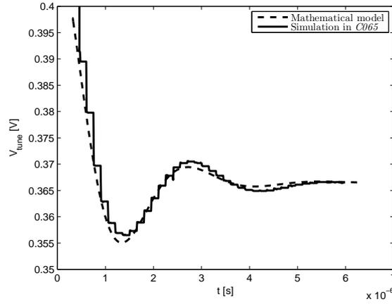
Figure 6.6: Verification of mathematical model through  $V_{tune}$  ( $R_{zero} < R_{opt}$ )
