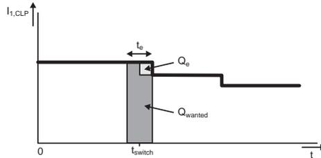
Figure 5.14: Reduced error in thermometer coded current source
