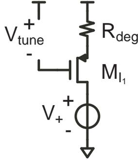
Figure 4.6: Current source  $I_1$  of the switched capacitor oscillator
