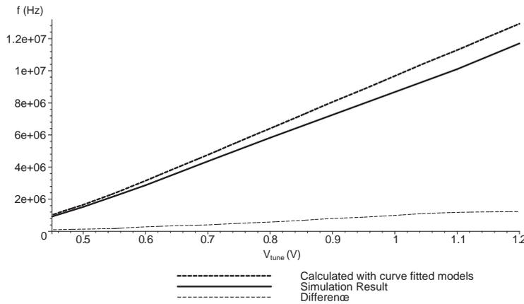
Figure 4.7: Frequency calculation curve fitted models for both  $I_1$  and  $M_1$
