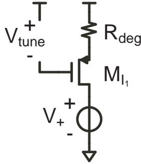
Figure 5.15: Degenerated current source
