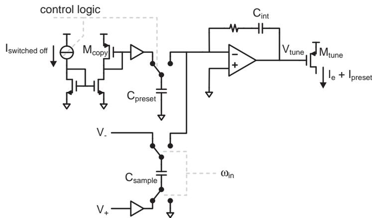
Figure 5.40: Presetting the integrator
