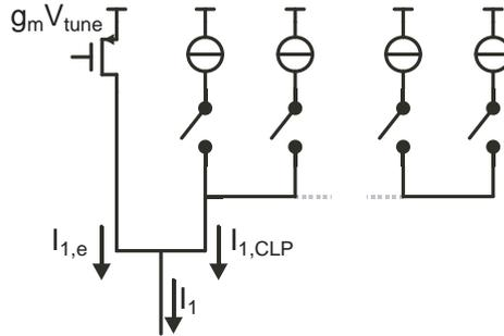
Figure 5.34: Semi-discrete current source  $I_1$
