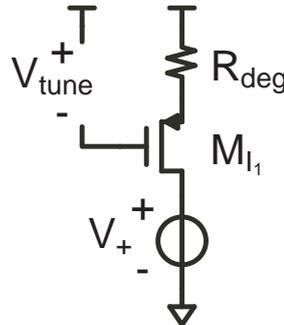
Figure 5.10: Current source  $I_1$  of the switched capacitor oscillator
