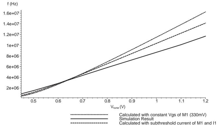
Figure 4.5: Frequency calculation with degenerated current source in subthreshold as well as  $M_1$
