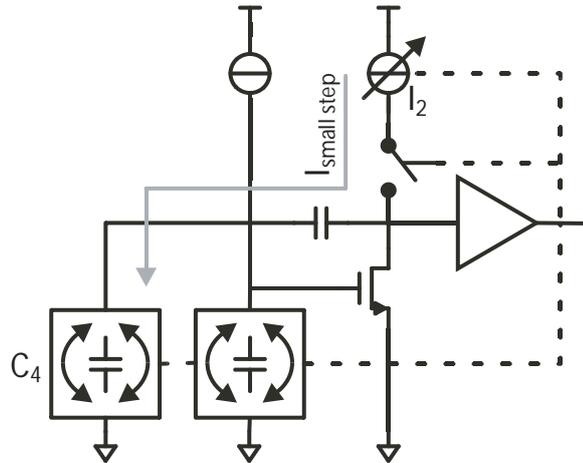
Figure 5.19: Small estimation step performed by an extra switched capacitor
