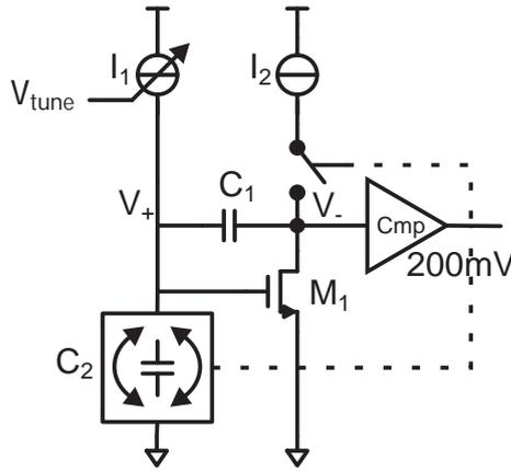
Figure B.1: Switched capacitor relaxation oscillator
