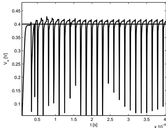
Figure 6.8:  $V_{GS,M_1}$ , and so  $V_+$ , stays around 400mV just before a capacitor is switched
