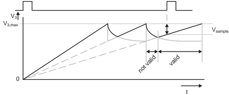
Figure 5.22: Time slots in which  $V_{sample}$  for the ML-Phase is valid or not
