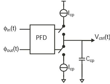
Figure 1.5: General charge-pump for a PLL
