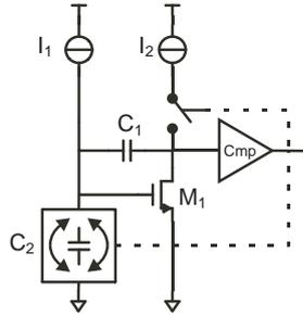
Figure 2.6: Switched capacitor relaxation oscillator
