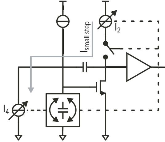
Figure 5.18: Small estimation step performed by extra current source(s)
