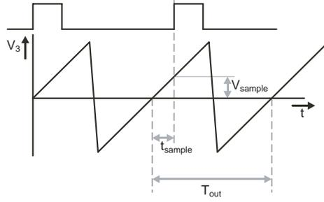
Figure 6.2: Graphical model of the PLL
