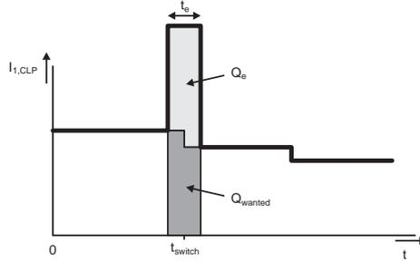
Figure 5.13: Error in binary coded current source during switching
