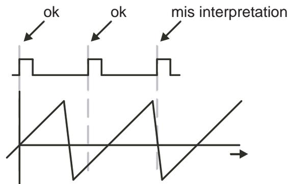
Figure 5.38: Misinterpretation of the excess phase
