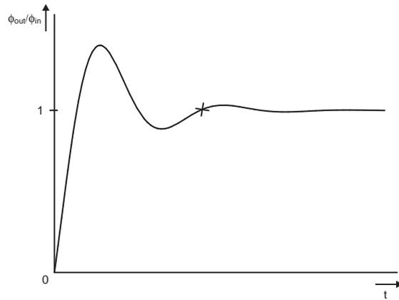
Figure 2.9:  $\phi_{out}/\phi_{in}$  starts from the cross due to integration of the frequency estimator
