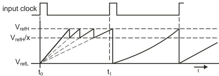
Figure 2.7: Integration of frequency estimator into relaxation oscillator
