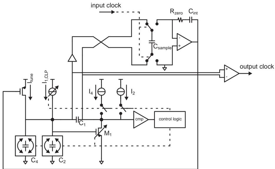
Figure 5.39: Circuit overview without the preset circuit and blocker
