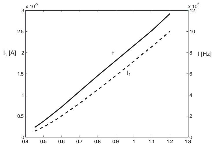
Figure 4.1: The frequency  $f$  (solid line) appears to be more linear than  $I_1$  (dashed line) as function of  $V_{tune}$
