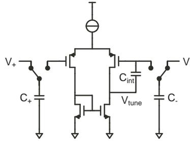
Figure 5.33: Differential to single-ended integrator to be implemented
