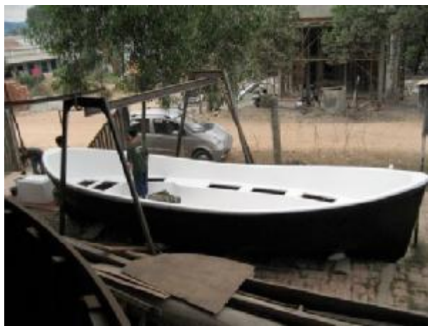
Figure 2 – Polyester lifeboat in production
