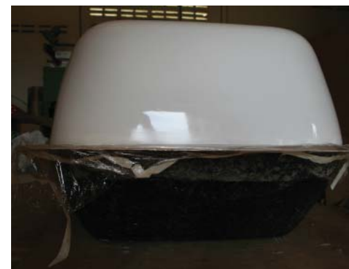
Figure F3: using plug and first mold part to produce the second moldpart
