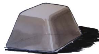
Step 1: produce the positive form. Grind well and polish carefully
