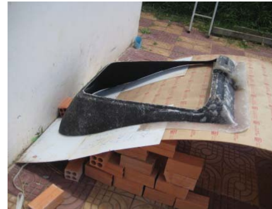
Figure F1: making flange using a curved foundation Figure F2: making flange using a stencil
