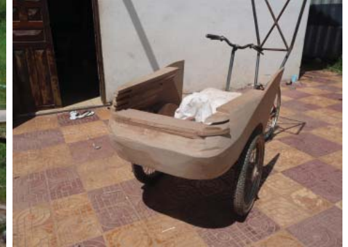
Figure A2: Glueing MDF to each other, layer for layer
