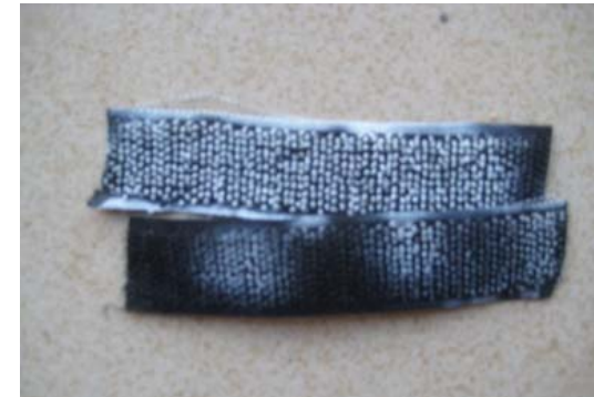
Figure L4: Super glue affecting the velcro straps
