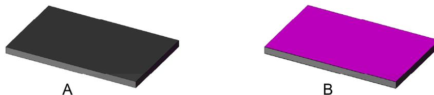
**Fig. 4-1: First process step, the deposition of SiRN. A: conductive silicon substrate. B: substrate insulated by the deposition of a 200 nm layer of SiRN (LPCVD).**
