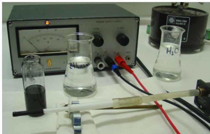
Figure 4.1: Rotated drying after dip molding, with the Ethanol and water ready for the phase separation.
