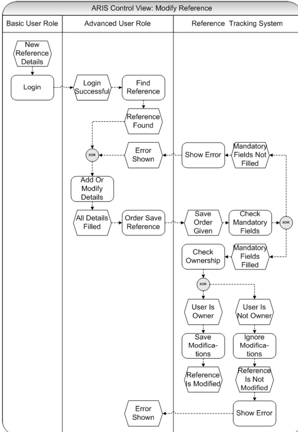
**Figure 23: Event-driven process chain diagram of modify reference process**
