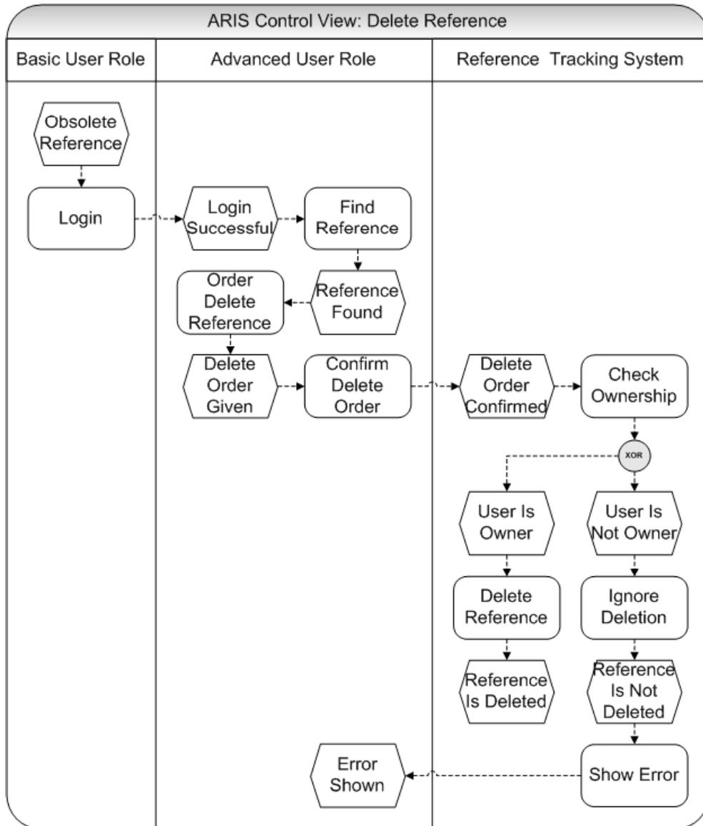
Figure 24: Event-driven process chain diagram of delete reference process
