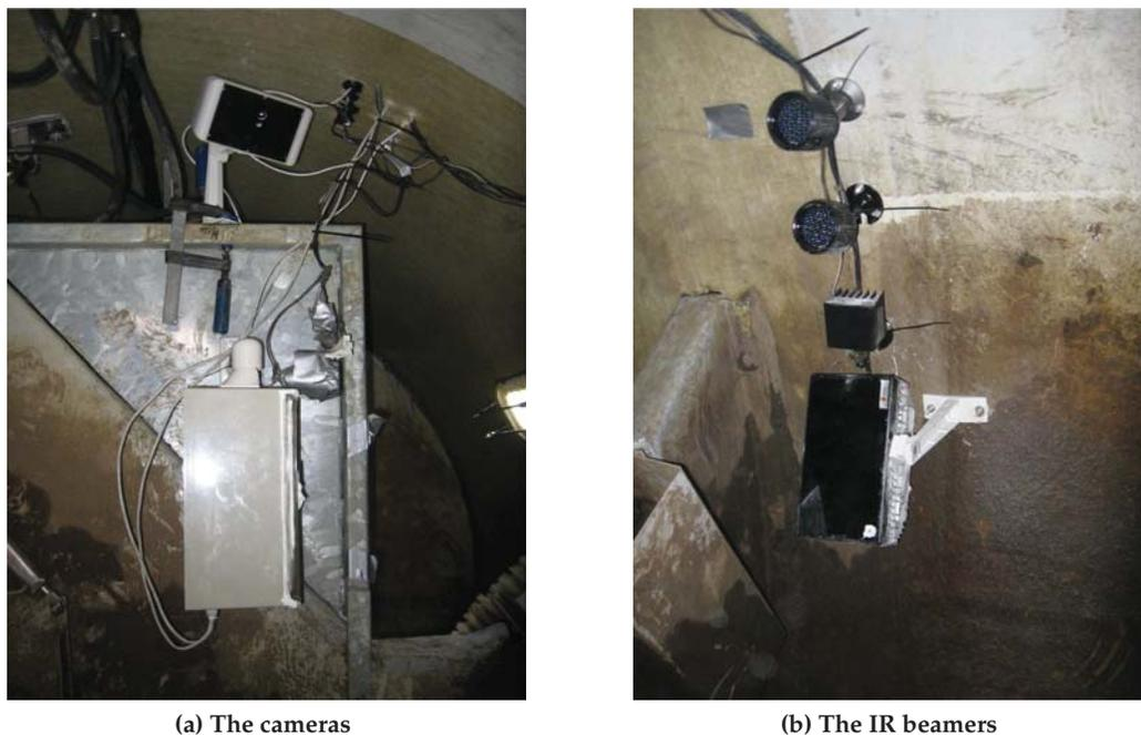
Figure 4.16: The cameras and IR beamers as used in the second setup.
