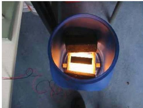
Figure 4.3: The setup used for obtaining images. A camera is placed above the barrel facing the partial covered light. At the moment of the picture there is no water in the barrel. During the experiment water is added to barrel. Every time 5 litre of water is added, this made a level raise of 5 cm, after this a new set of pictures is taken with the camera above the barrel.
