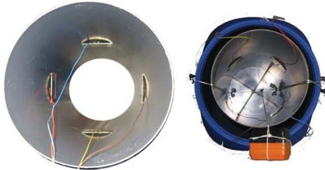
Figure 5.23: The tube with the electrodes as used for the experiment (left) with a closed bottom and placed inside a barrel (right)
