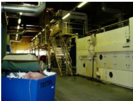
Figure 6. Hotflue of the pre-dyeing machine after the IR-dryer [12]
