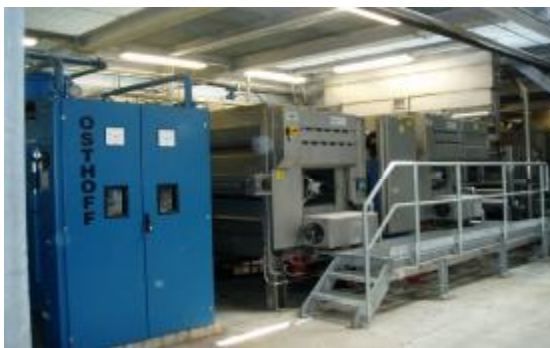
Figure 1. Singeing machine and impregnation bath of the desizing step of the CBB [12]
