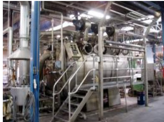
Figure 5. Discontinuous dyeing machine (jet) [12]
