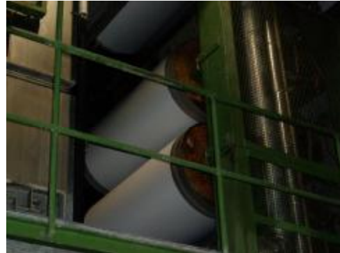
Figure 2. Steam-heated drying cylinders [12]
