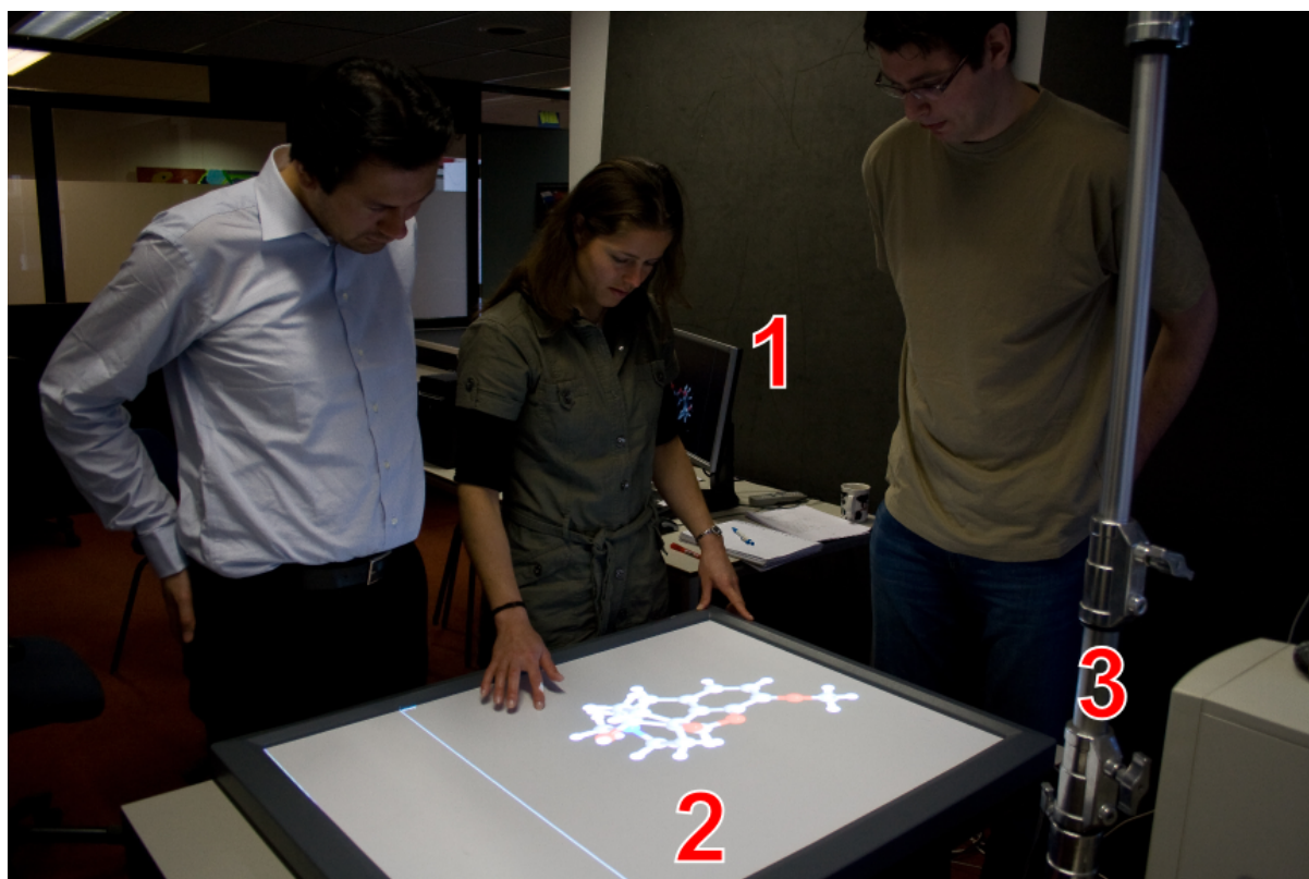
Figure 1.1: Hardware setup of TouchMol. Taken during a user test, this figure shows the PC (1) running TouchMol, which is projected onto the DiamondTouch table (2) using the projector suspended from a stand (3).
